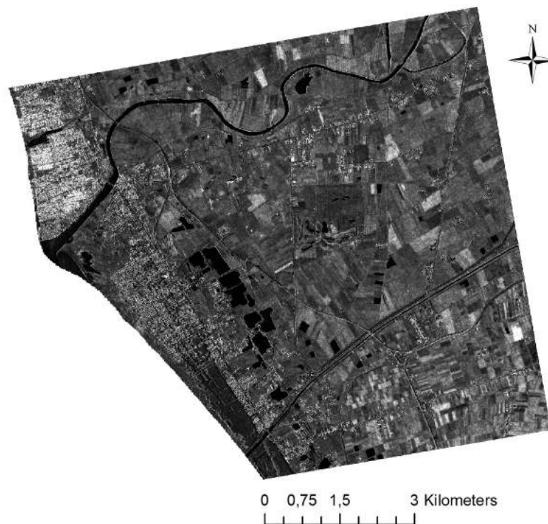
Figure 2. One of the available SAR images in amplitude format. The area is about 14 \times 12 \text{ km}^2 with a spatial resolution of 3 m/pixel.
