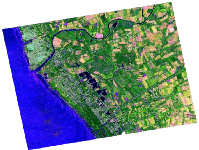
Fig. 4: Campania dataset, summery Level-1 \beta product obtained by processing eight images from April to October 2010. Roughly, the following color-object association can be made: blue-sea, black-stagnant water/weak scatterers, green-grasslands/unchanged land cover, cyan-built-up, yellow/pink-growing vegetation. The original image dimension is about 4400 \times 5000 pixels.
