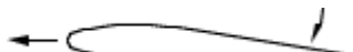
The air is pulled forward as well as down by the motion of the wing.
