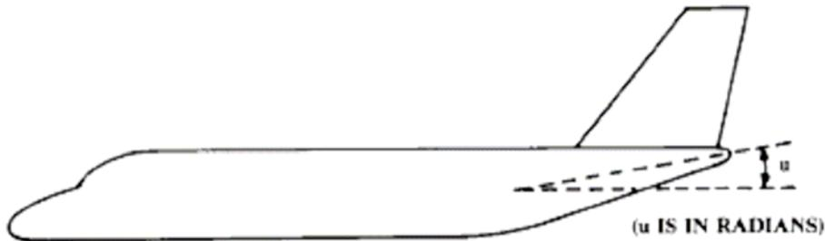
**Fig. 12.24 Fuselage upsweep.**
