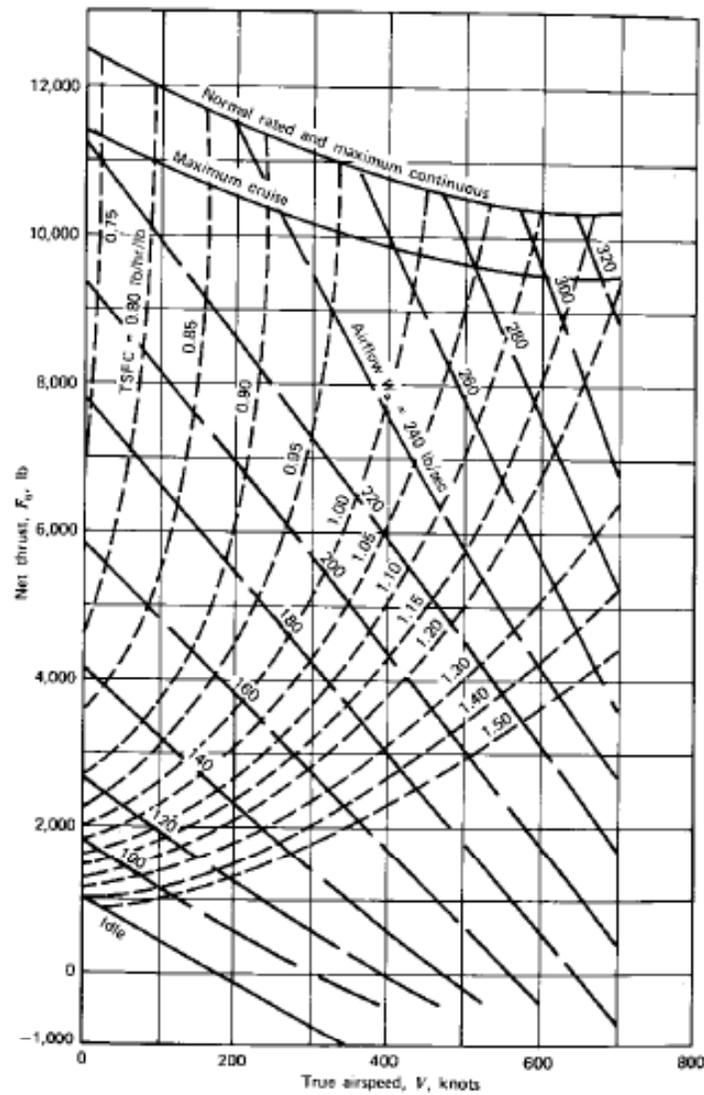
**Figure 6.32a** Pratt & Whitney Aircraft JT4A-3 turbojet engine. Estimated thrust, TSFC, and airflow at sea level. Standard atmospheric conditions, 100% ram recovery. (Courtesy, Pratt & Whitney.)
