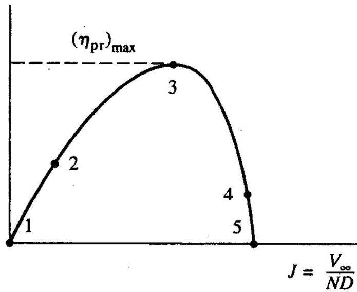
(a) Propeller efficiency
