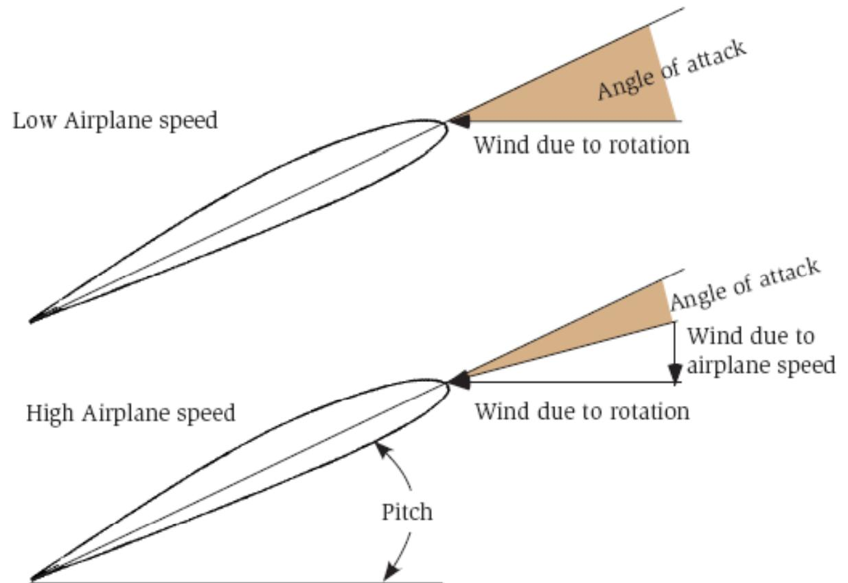
Fig. 5.5. Angle of attack of a rotating propeller.
