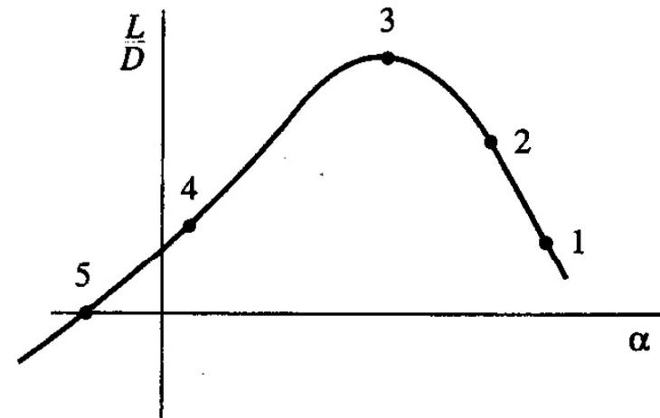
(b) Lift-to-drag ratio of a given propeller airfoil cross-section
