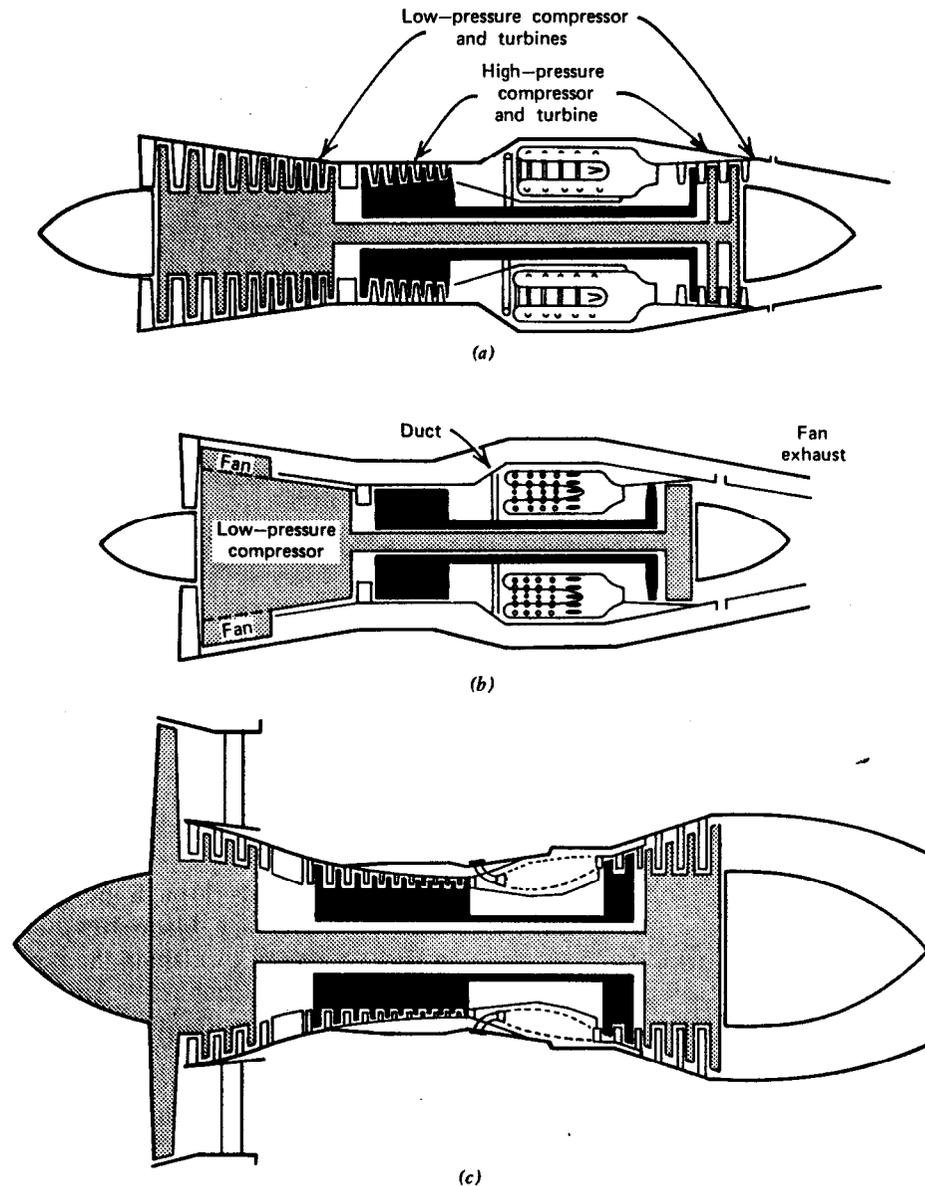
**Figure 6.26** Variations on the gas turbine. (a) Dual axial-flow compressor turbojet. (b) Dual axial-flow compressor, forward fan engine with long ducts. (c) High bypass ratio turbofan with short ducts. (d) Single axial-flow compressor, direct propeller drive turboprop. (e) Single axial-flow compressor, free turbine propeller drive turboprop. (f) Dual axial-flow compressor, turbojet with afterburner. (g) Dual axial-flow compressor, industrial turboshaft engine.
