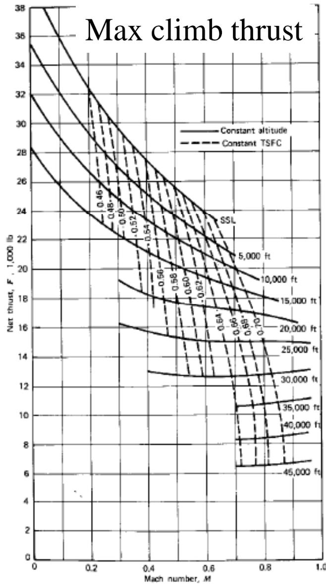
**Figure 6.37** JT9D-7A maximum climb thrust. One hundred percent ram recovery, no airbleed, no power extraction, Pratt & Whitney Aircraft reference exhaust system, all curves for ICAO standard day +10°C and below. (Courtesy, Pratt & Whitney.)
