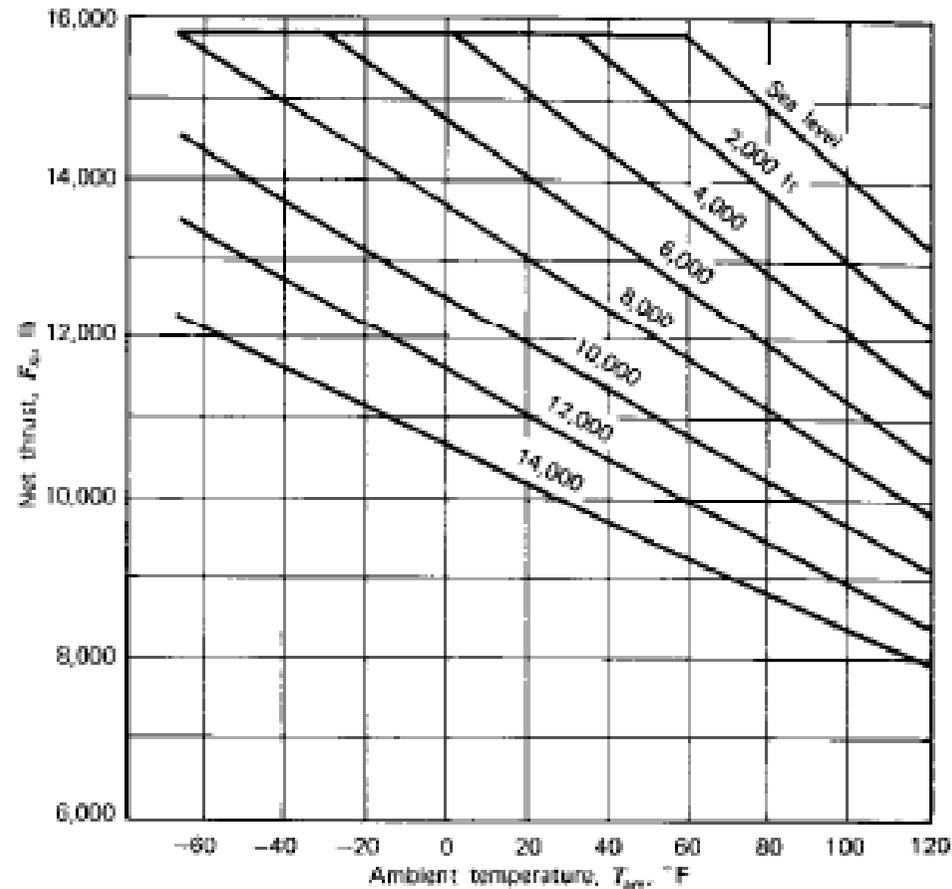
**Figure 6.33a** Pratt & Whitney Aircraft JY4A-3, -5 turbojet engines. Estimated net thrust on runway during takeoff. Zero knots. (Courtesy, Pratt & Whitney.)
