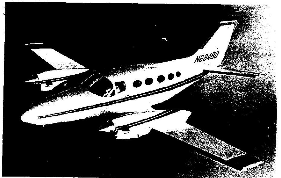
Cessna Conquest I six/eight-seat twin-turboprop pressurised transport
