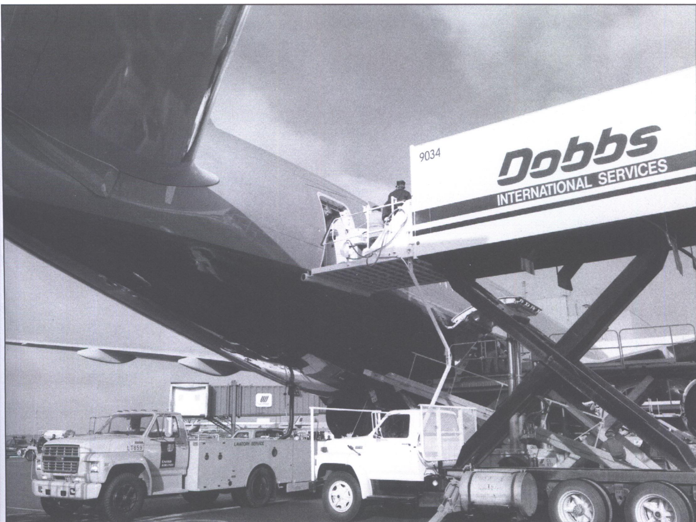
Galley truck and lavatory service truck during a fit check on WA004 at Seatac airport, Washington December 18, 1994. Notice how the various functions can occur simultaneously. (Boeing/Brett Olson)
