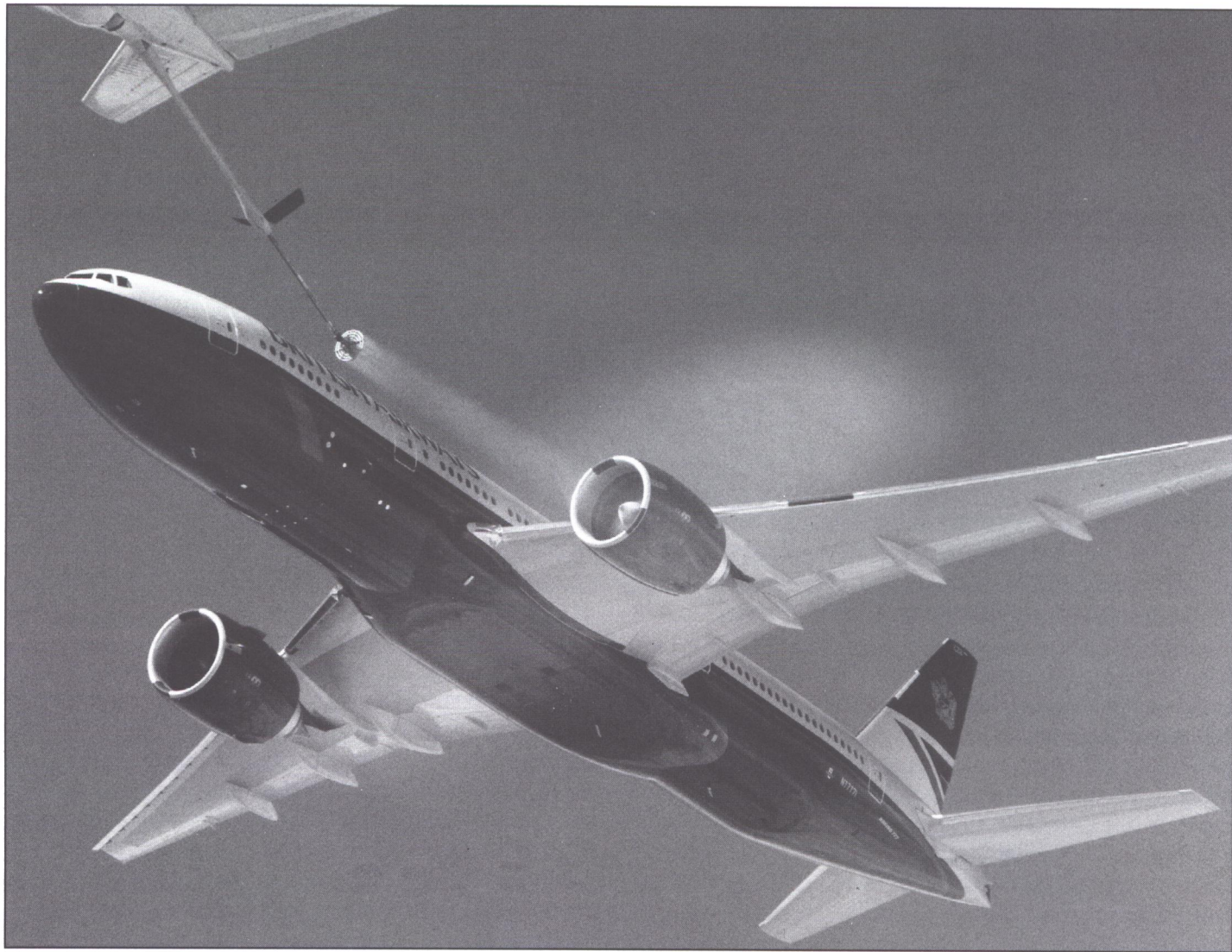
During icing tests behind the KC-135 tanker, water spray forms an ice cloud. The ice cloud is the result of the correct combination of cold temperature at altitude, and the controllable water droplet size from the tanker. (Boeing/Jeff Rumsey).
