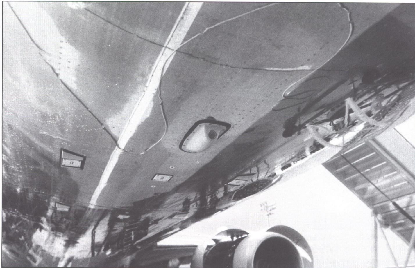
Ground maneuver camera on the bottom of the fuselage and aft of the nose gear. The line and cable are a reflection of items on the ground in the highly reflective aluminum. This is the first production aircraft use of a ground maneuver camera system. (Author)
