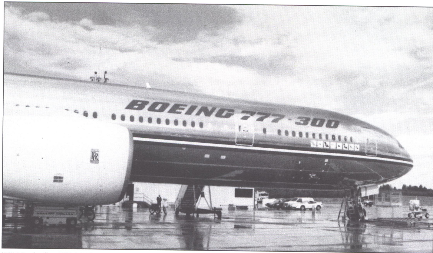
WB501, the first 777-300, is powered by Rolls-Royce Trent 892 engines. Two more flight test aircraft will be Rolls-Royce powered and another three will be Pratt & Whitney powered. (Author)
