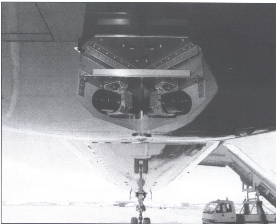
Instrumentation cameras located on the bottom of the fuselage of WA001. These cameras were used during the rejected takeoff tests at Edwards Air Force Base, California. (Boeing/ Brett Olson)
