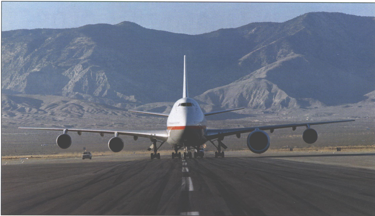
GE's 747 flying testbed with the GE90 engine on the left inboard position, ready for take off at Mojave, California. Notice the small amount of ground clearance, which is only 13 inches, on the test engine for the 777. (GE Aircraft Engines)
