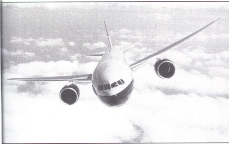
Boeing 777 twinjet powered by GE90 engines. The impressive size of the engines compared to the wide-body fuselage is evident in this head on, in-flight view. (GE Aircraft Engines)
