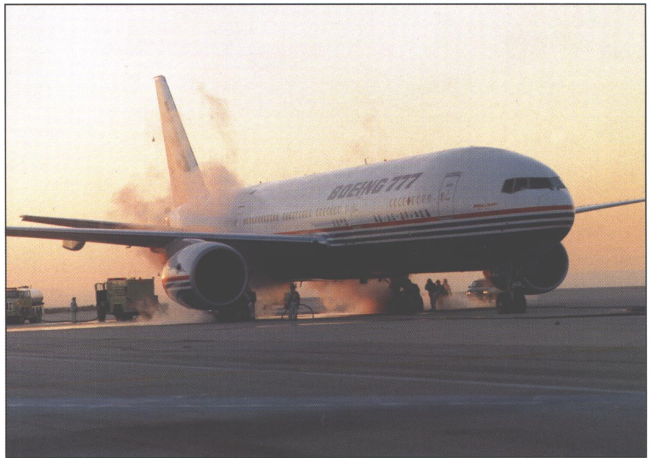
Fire department cools down the 3000 degree red-hot brakes at the end of the 100 percent RTO test at Edwards Air Force Base in California. 14,000 gallons of water are applied to the brakes and deflated tires after waiting five minutes to simulate normal response time. (Boeing)
