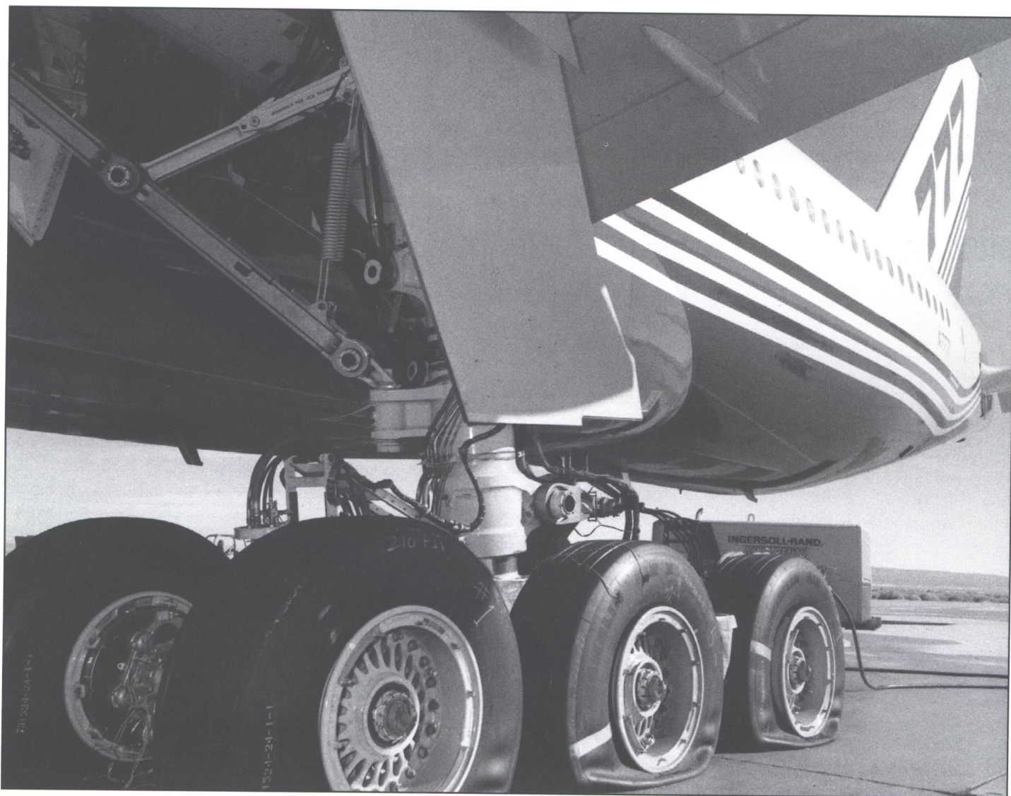
Before the tires explode from the heat induced pressure build-up at the end of the RTO test, safety fuse plugs on the tires blow. Tires, wheels, and brakes are literally destroyed in this test. (Boeing/Brett Olson)
