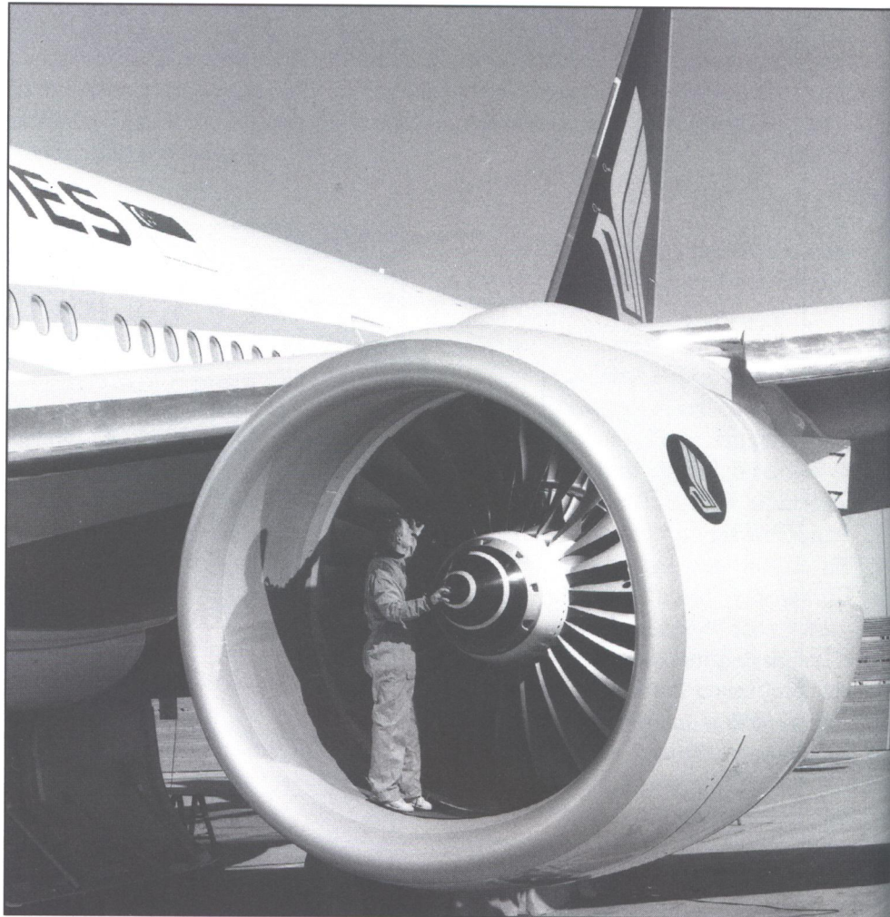
Singapore Airlines Rolls-Royce Trent 800 powered 777. The massive size of the turbofan engine is apparent with the technician standing in the inlet. (Rolls-Royce)
