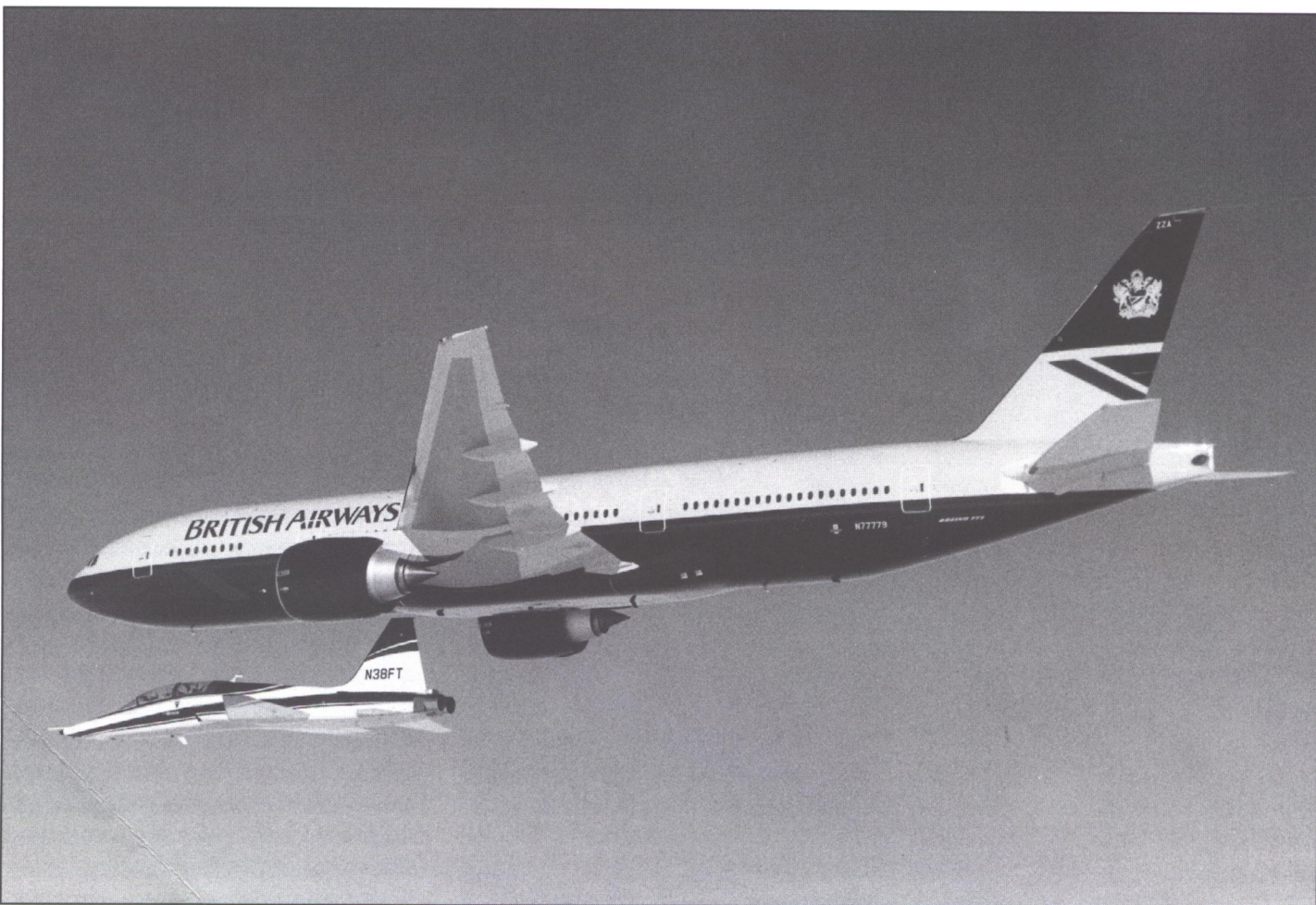
T-38 chase aircraft with N7779, the first British Airways 777, during flutter tests with GE engines, February 17, 1995. Each engine-airframe combination for the three different engine options requires a complete set of tests. (Boeing/ Debra O'Brezar)
