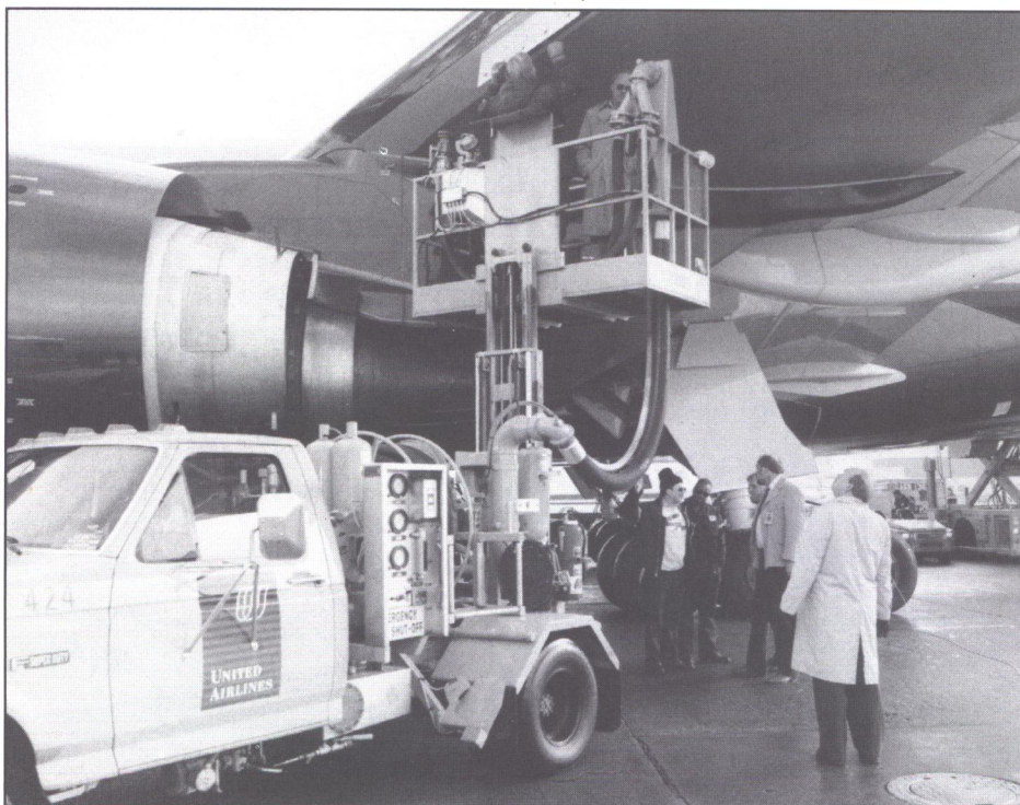
Fueling from a hydrant fuel truck, which provides the connection between the underground fuel system and the aircraft. The main difference between the hydrant fuel truck and the standard fuel truck is that the hydrant truck carries no fuel. (Boeing/Brett Olson)
