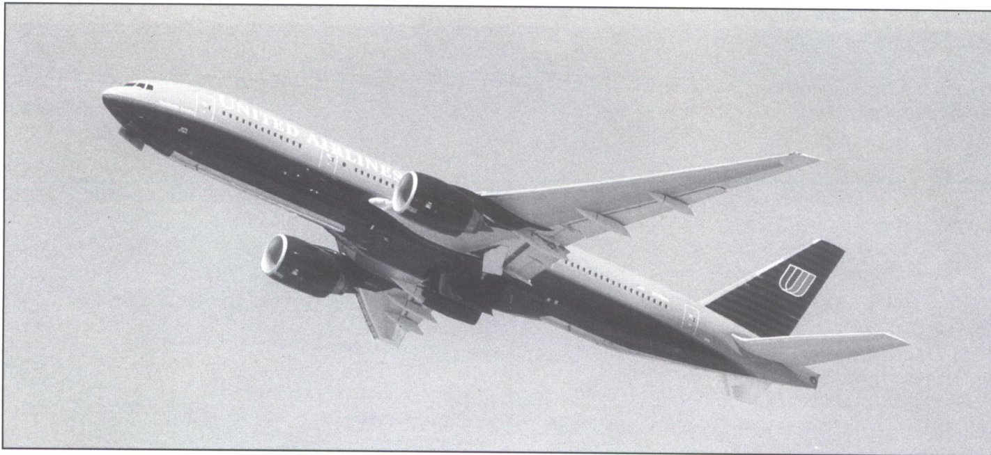
A United 777 take-off from Los Angeles with landing gear doors almost closed. Closing the doors once the landing gear is extended reduces drag until it is time to retract the gear. (Stephen Griffin)
