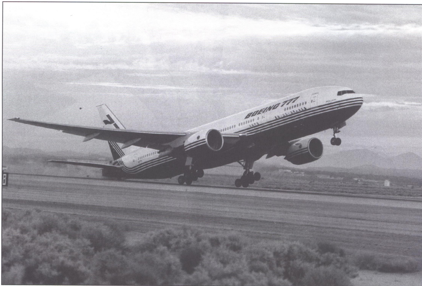
Tail dragging during VMU tests at Edwards Air Force Base on September 15, 1994. The Velocity Minimum Unstick tests are conducted to determine the aircraft's minimum takeoff speed. This test requires the aircraft's tail to come in contact with the runway prior to takeoff. (Boeing/Bob Carnahan)
