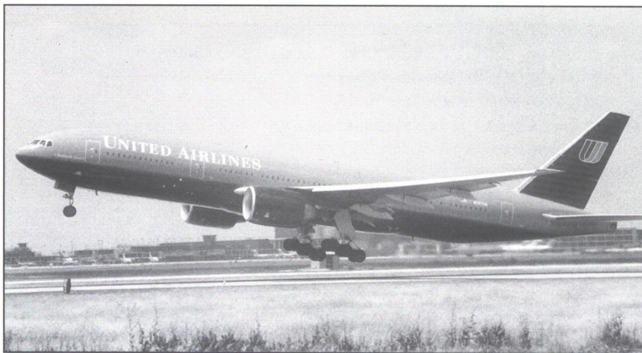
N767UA taking off from Chicago O'Hare airport, July, 1996. Notice the 13 degree tilt of the six wheel main landing gear. (Tom Pesch)
