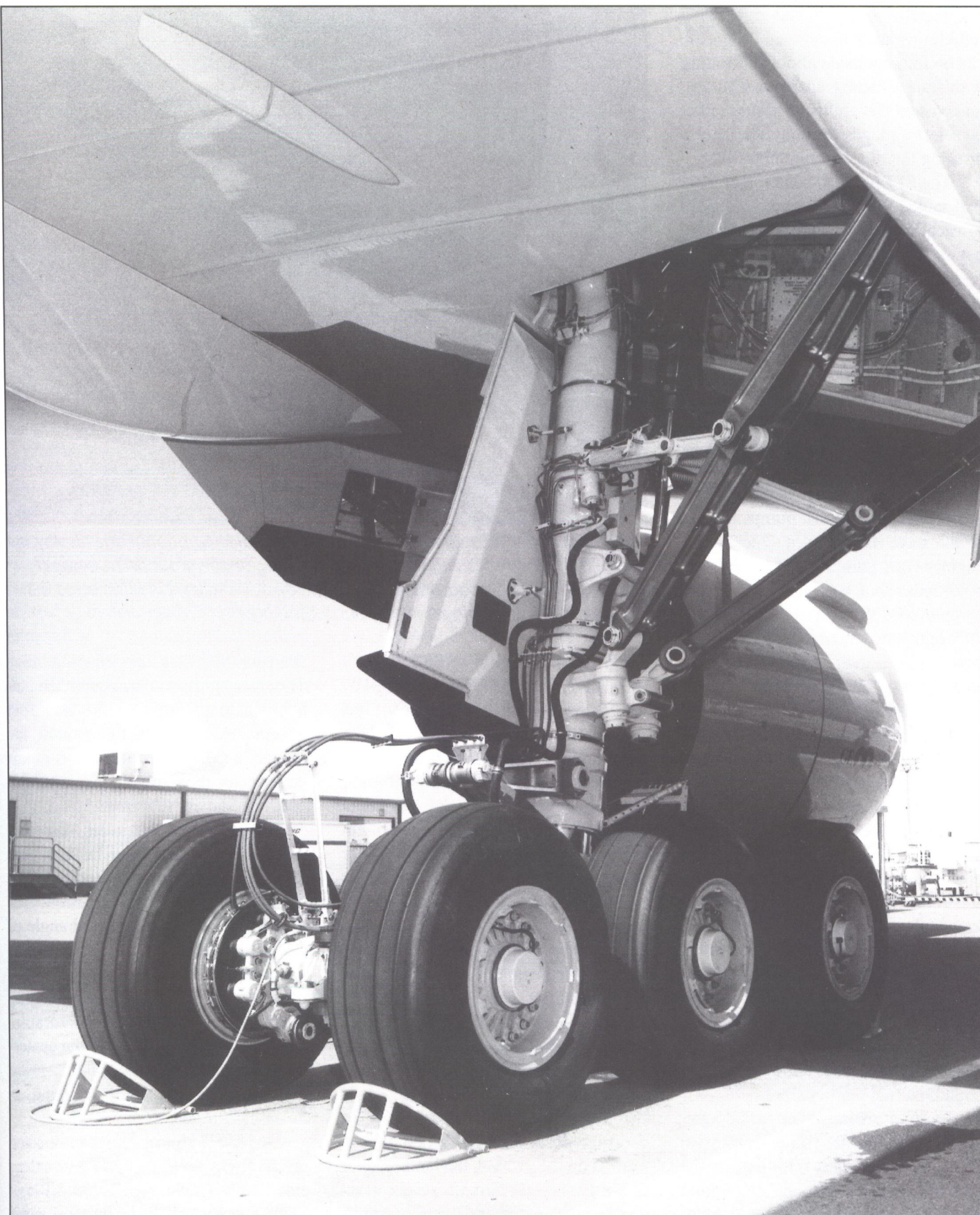
The unique three-axle six-wheeled main landing gear on the 777. The landing gear truck is tilted up 13 degrees when extended in flight and moved to a five degree down position for retraction. (Boeing)
