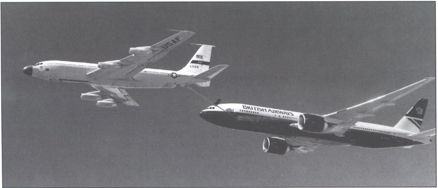
U.S. Air Force KC-135 tanker during icing tests on WA077, October 6, 1995. This specially modified KC-135 based at Edwards Air Force Base, California, carries large water tanks in the fuselage and uses a special controllable spray nozzle in place of the normal refueling probe. (Boeing/Jeff Rumsey)
