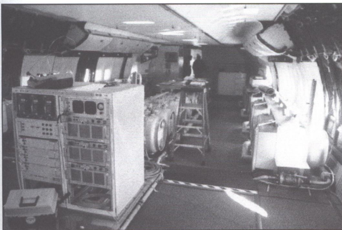
Forward water ballast and instrumentation racks in WB 501. Partial cabin trim and luggage compartments have been installed in the first flight test aircraft. (Author)
