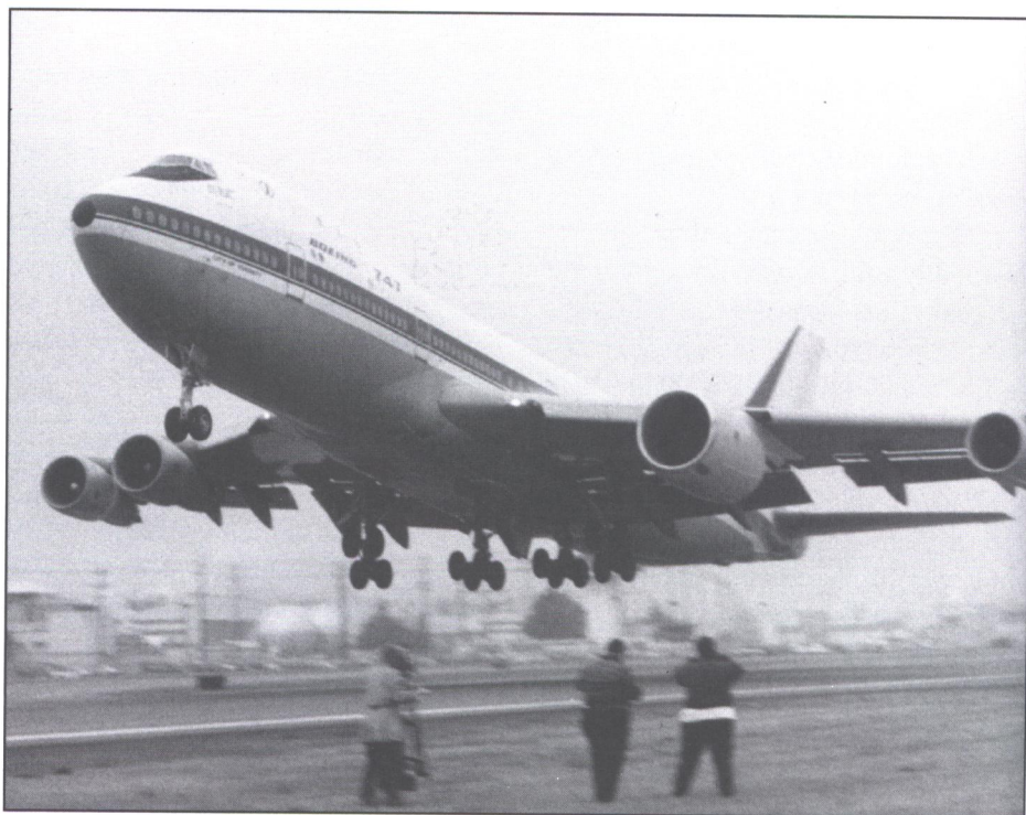
Boeing's 747 flying testbed takes off with Pratt & Whitney's PW4084 mounted on the left inboard pylon. A total of seventeen flights and 56 hours were flown with the P & W engine on the Boeing 747 flying test bed. (Pratt & Whitney)
