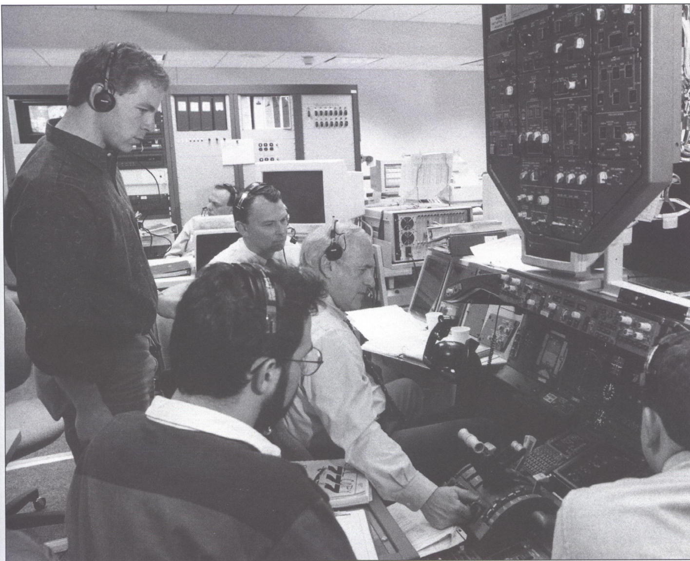
Systems Integration Lab (SIL) was so complete, it was often referred to as "airplane zero". Here Capt. John Cashman, chief pilot (center), prepares for a "takeoff". SIL testing started 13 months before the first flight of the 777. (Boeing)
