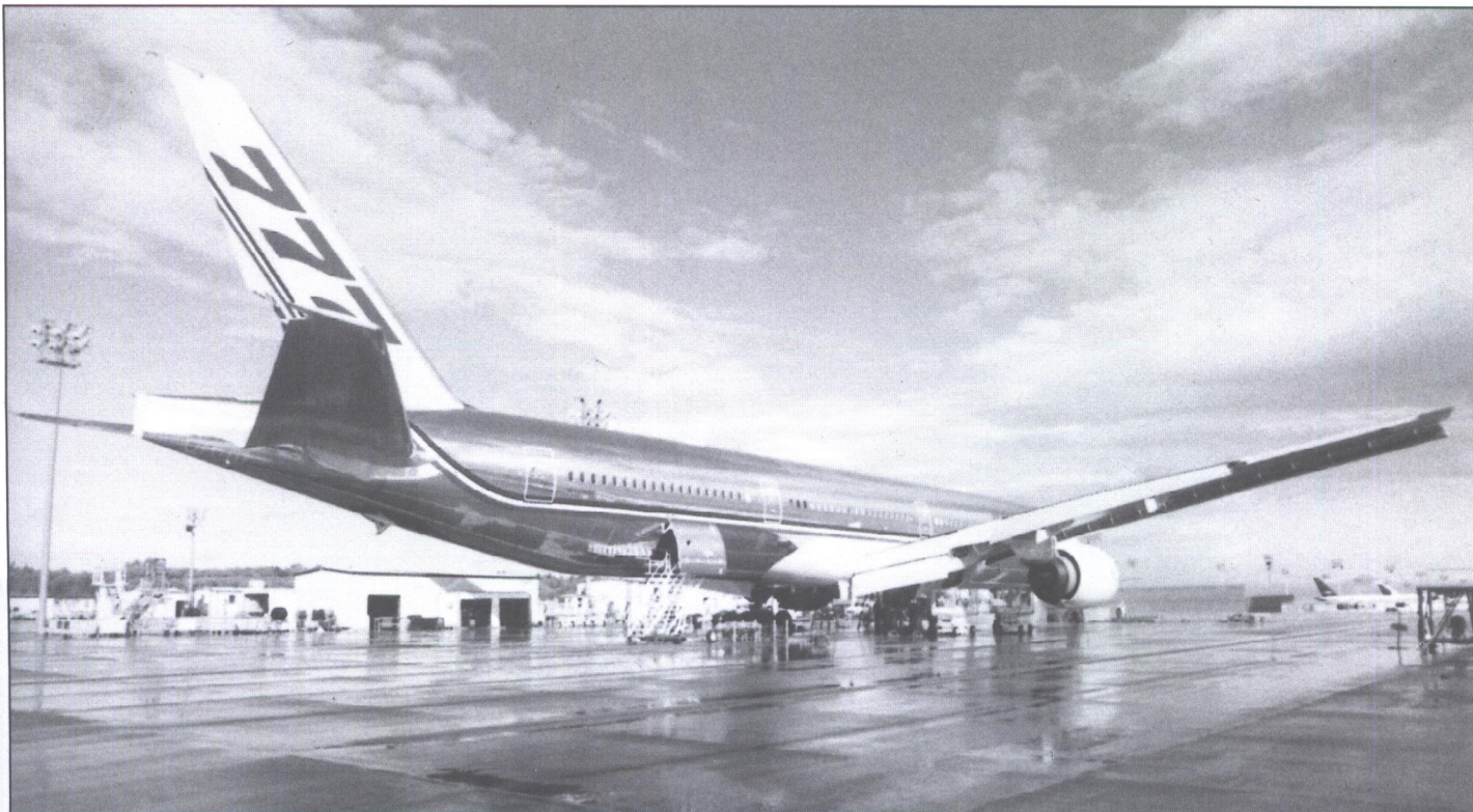
Long length of the -300 is evident in this view. Flat shape of the tail cone, which houses the APU, is still a distinguishing feature for identifying a 777. The additional door over the wing is a method of identifying a -300. (Author)
