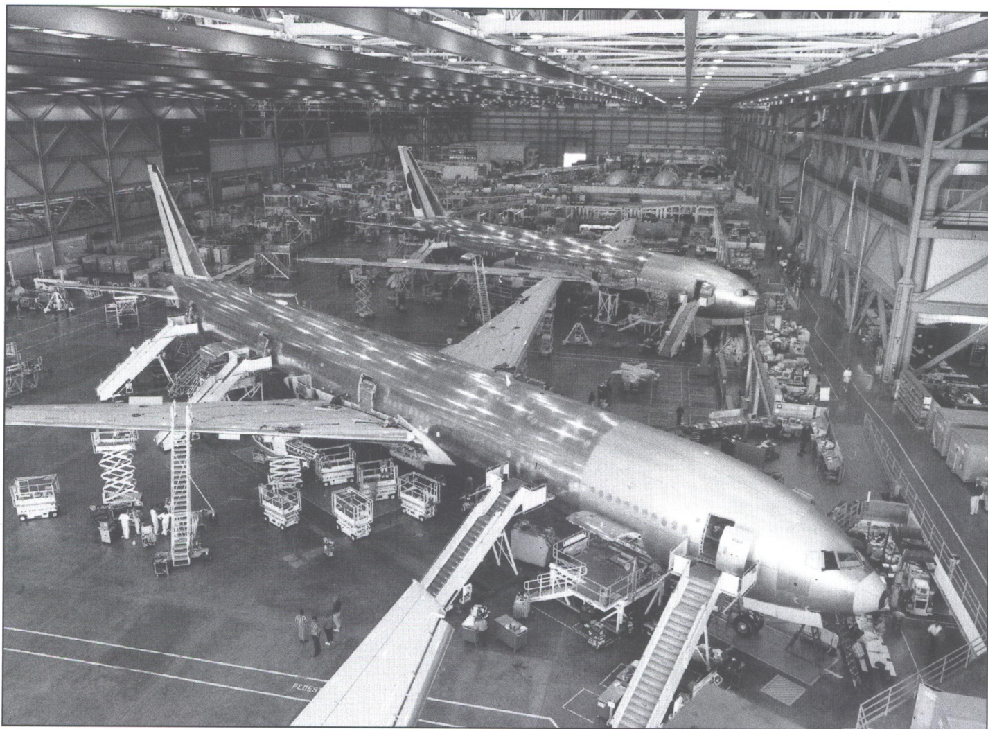
First 777-300 in the final assembly position, where engines and the APU are installed and functional checks are run on the aircraft systems. Notice the additional door position over the wing. (Boeing)
