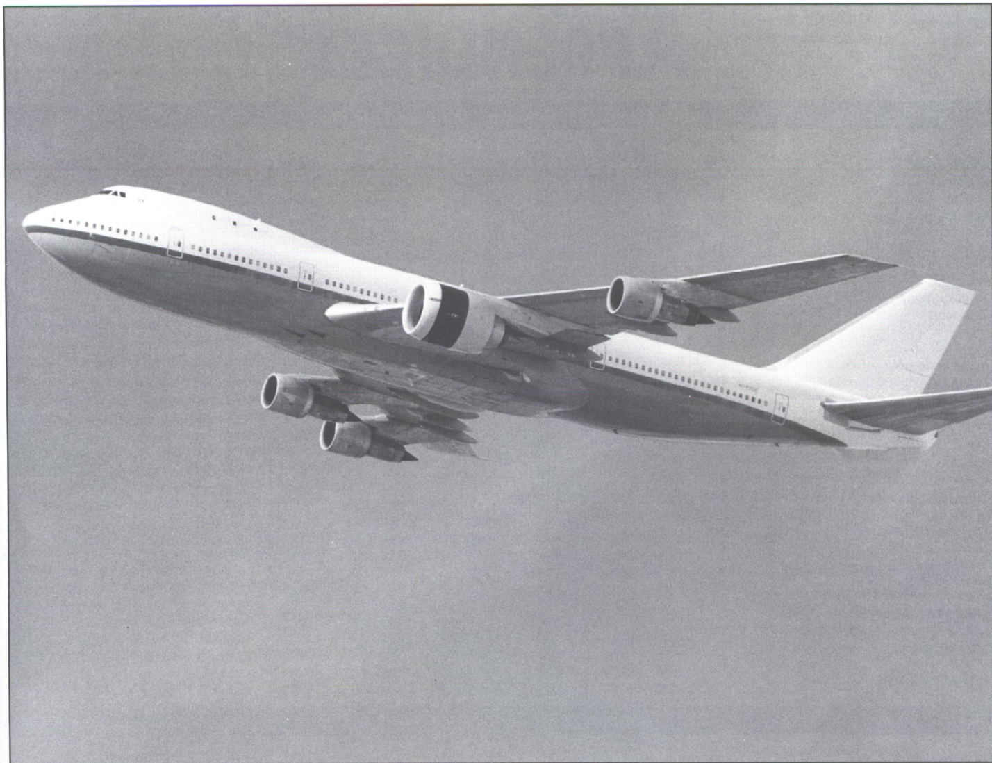
Engine flight testing of a GE90-92B, mounted on the inboard location on the left wing of the GE 747 flying testbed. This is a 92,000 lb thrust version of the GE90 engine. (GE Aircraft Engines)
