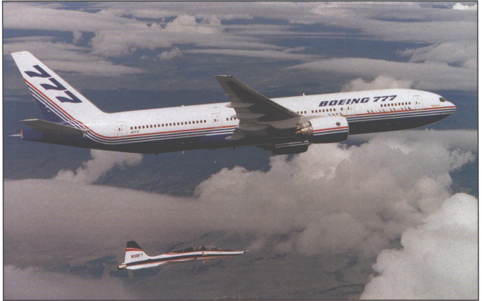
First flight of the Boeing 777-200 on June 12, 1994, flown by Capt. John Cashman, 777 chief pilot, and Capt. Ken Higgins, director of Flight Test for Boeing. The Northrop T-38 chase aircraft belongs to Boeing Commercial Airplane Group Flight Test and is used on first flights and critical high speed and flutter tests where an external observer is essential. (Boeing)
