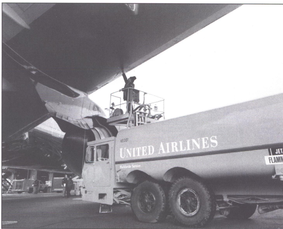
Fueling from a standard fuel truck under the right wing during a fit check demonstration on WA004 at Seatac Airport. The right wing refueling station is an option in addition to the left wing station. Both left and right stations can be used at the same time, offering faster refueling times. (Boeing/Brett Olson)
