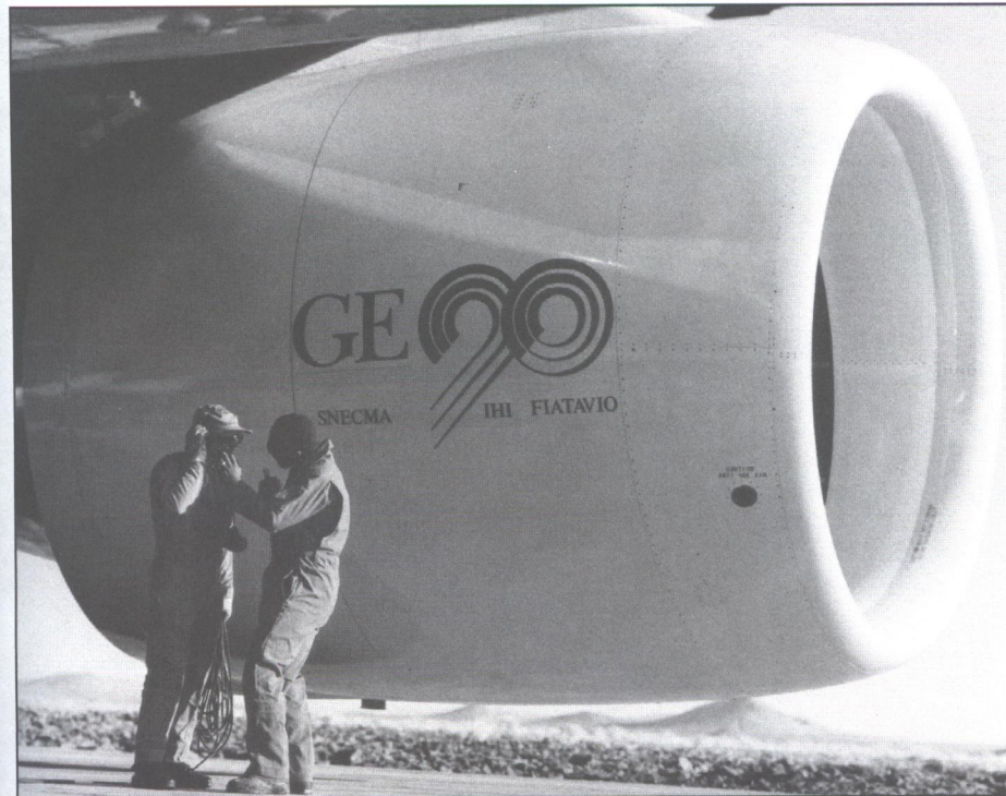
GE90-85B flight test engine mounted on the 747 flying testbed at Mojave California. Notice the ground clearance on this enormous engine. (GE Aircraft Engines)
