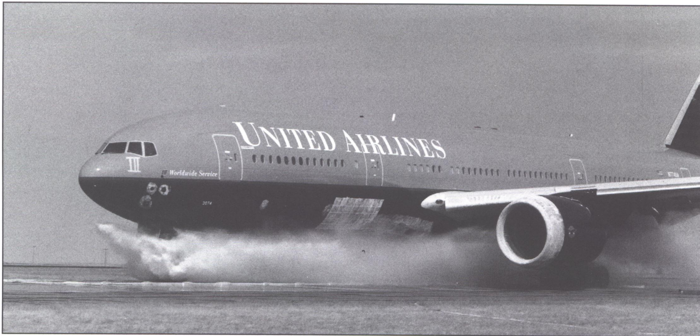
Water spray ingestion testing is accomplished at Glasgow, Montana on July 30, 1994, on WA002. The nose gear is run through a trough of water to evaluate effects of the water spray ingestion. (Boeing/ Joe Parke)
