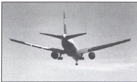
United Airlines 777-200 landing at Chicago O'Hare, September 1996. Bulge on the bottom of the fuselage, where the landing gear wheel well is located, can be seen in this view. Notice that the landing gear doors are closed after the gear has been extended. (Tom Pesch)
