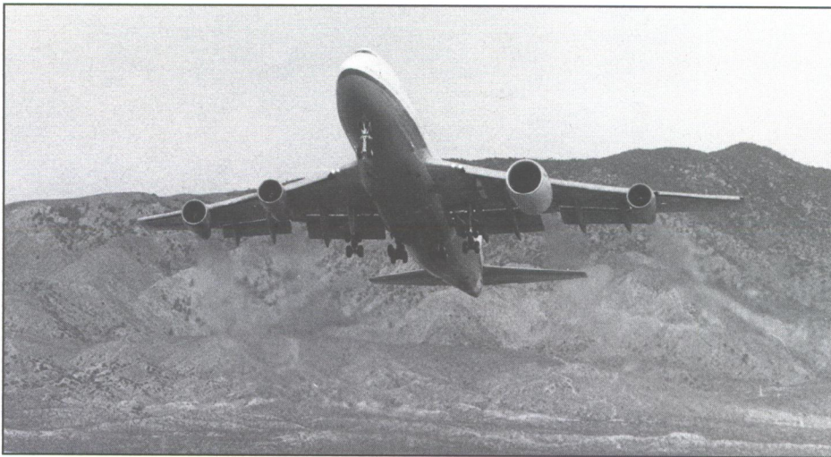
Engine flight testing of a GE90-85B engine, mounted at the inboard location on the left wing of GE's 747 flying testbed. The data collection system on board the test bed has the capability to record 3000 measurements. Typical crew size during test flights ranges from 16 to 25. (GE Aircraft Engines)
