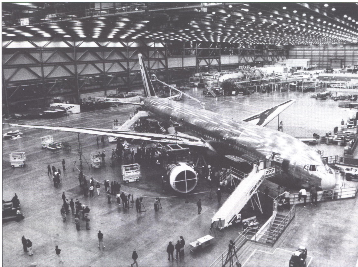
PW4084 engines being installed on the 777. Engine installation occurs at the final assembly position of the production line. United Airlines was the launch customer for the Pratt & Whitney engines, and the initial launch customer for the 777. (Pratt & Whitney)
