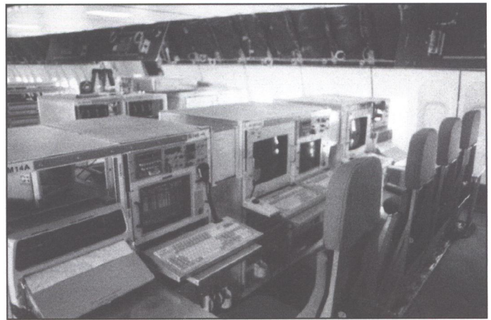
Flight test airborne data system in the -300. Consoles are used for in-flight monitoring and analysis of the flight test data. (Author)
