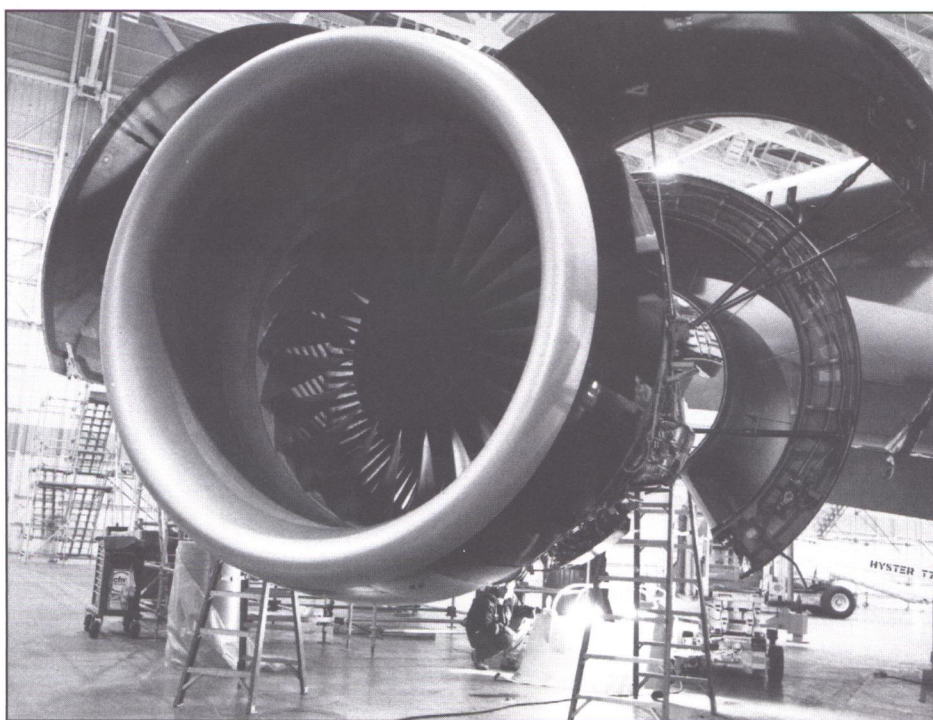
PW4084 engine on 777 WA003 with the engine cowl doors open. The first five aircraft built, WA001 through WA005, were all powered by P&W engines. (Boeing/Bob Carnahan)
