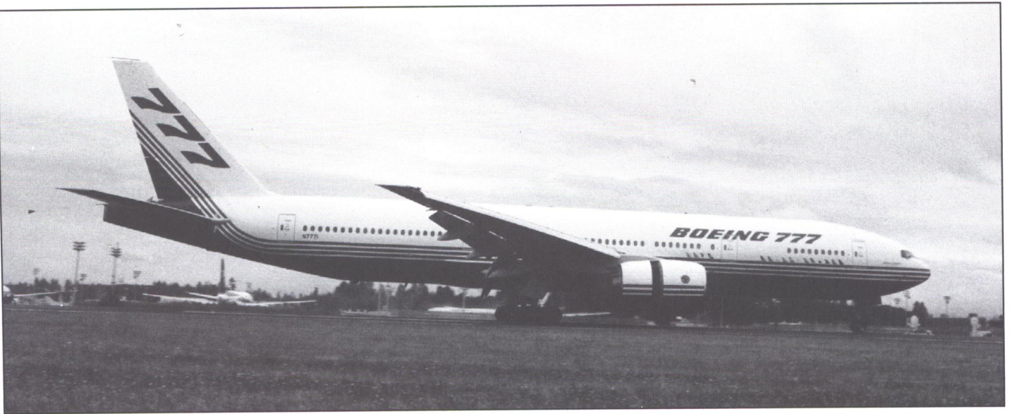
Landing from first flight under cloudy skies at Paine Field, Everett, Washington. Note the thrust reversers in use. All tests went well. Pilots reported exceptional trim and excellent handling qualities. (Boeing/Denise Blangy)
