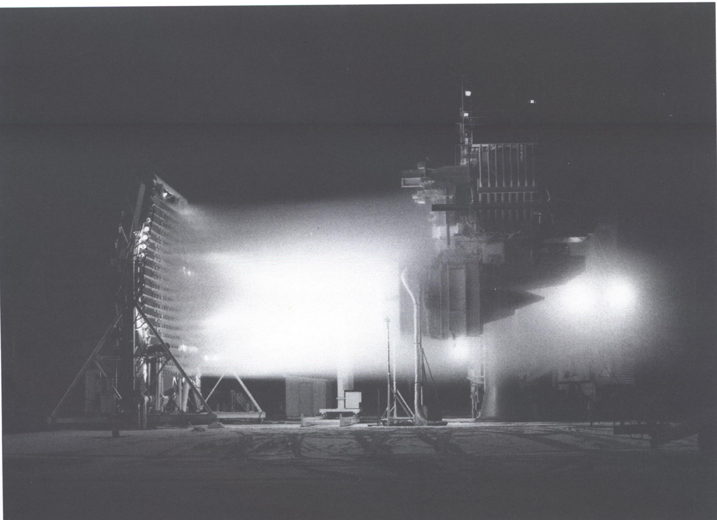
Icing tests, in this spectacular night photo of a GE90 high bypass turbofan engine, are representative of the testing that is done prior to flight and for future development models of the GE90 engines. (GE Aircraft Engines)
