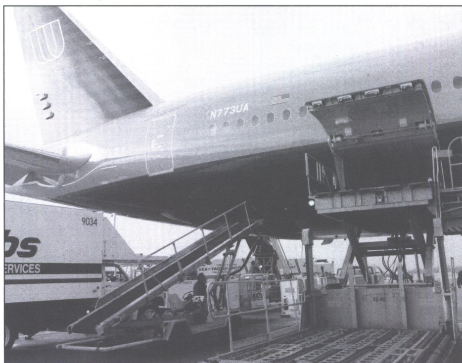
Galley truck and lavatory service truck during a fit check on WA004 at Seatac airport, Washington December 18, 1994. Notice how the various functions can occur simultaneously. (Boeing/Brett Olson)
