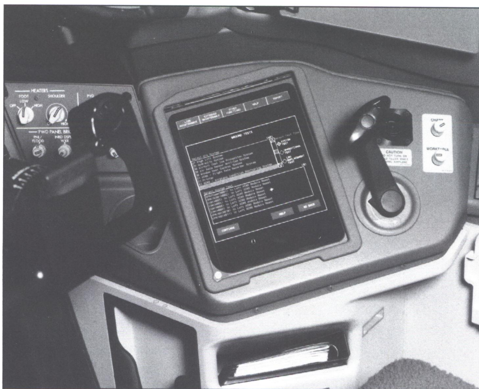
The steering tiller, located to the right of the first officer's optional side display, is one of the flight deck steering controls for taxiing on the ground. The captain's tiller is on the left outboard side of the flight deck. The tiller is in addition to the rudder pedals for steering on the ground. (Boeing)
