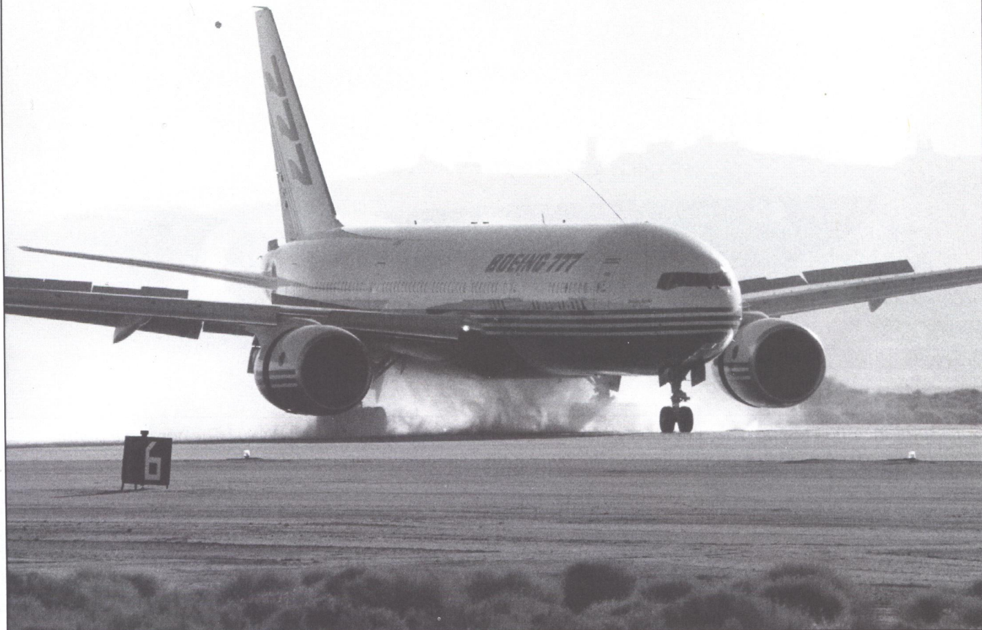
Wet runway tests, simulating adverse weather runway conditions, are used to check aero performance and braking. Edwards Air Force Base water tankers have applied 27,000 gallons of water on the desert runway. (Boeing)
