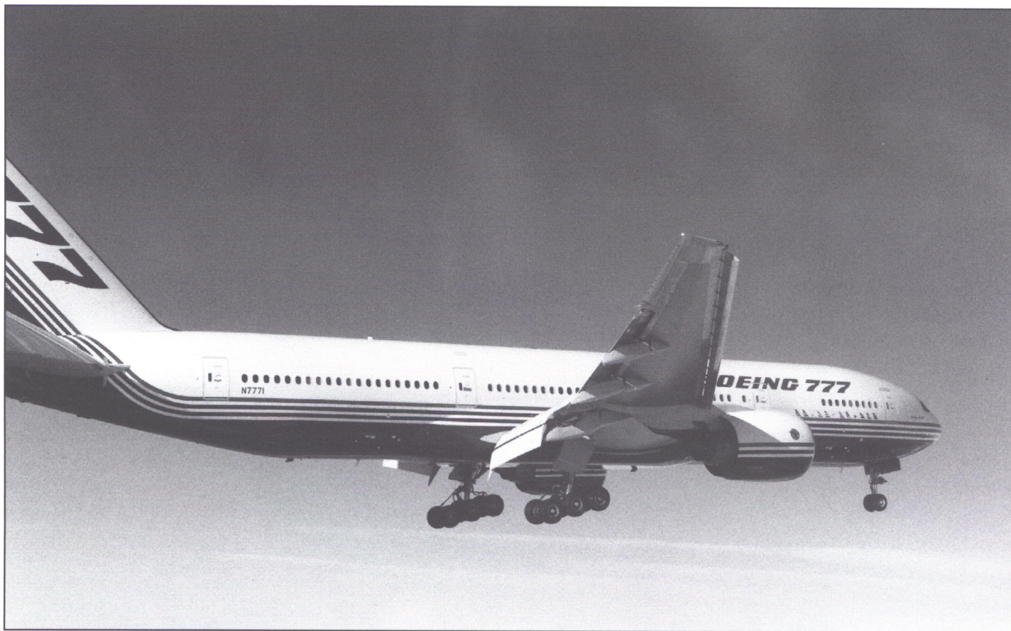
A good photo showing the flaps and leading edge slats deployed to the high lift position with the aircraft in slow flight and the landing gear down. The High Lift Control System (HLCS), an electronic fly-by-wire system, has inboard and outboard trailing edge flaps, leading edge slats, and Krueger flaps. (Boeing/Jeff Rumsey)
