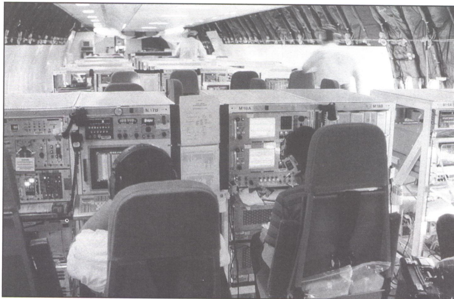
Data systems in operation on the 777. Typical crew size during these flights ranges from 8 to 25. (Boeing)
