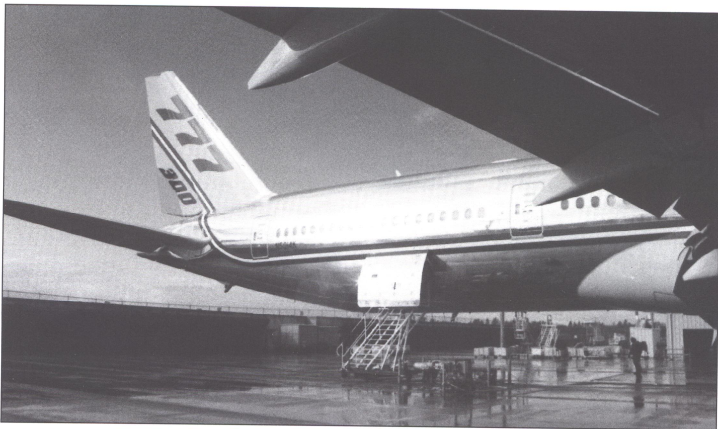
Aft fuselage view of WB501 during preflight preparation. Flap mechanism fairings can be seen at the top of the photo. (Author)
