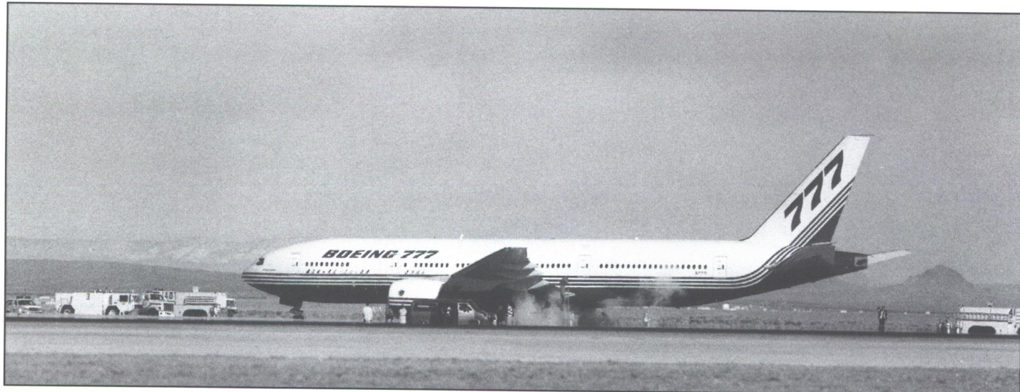
Fire trucks stand by at the end of the 100 percent Refused Takeoff (RTO) test at Edwards Air Force Base California on Jan 31, 1995. Brake temperatures reach 3000 degrees and get red hot during this test. (Boeing/ Brett Olson)
