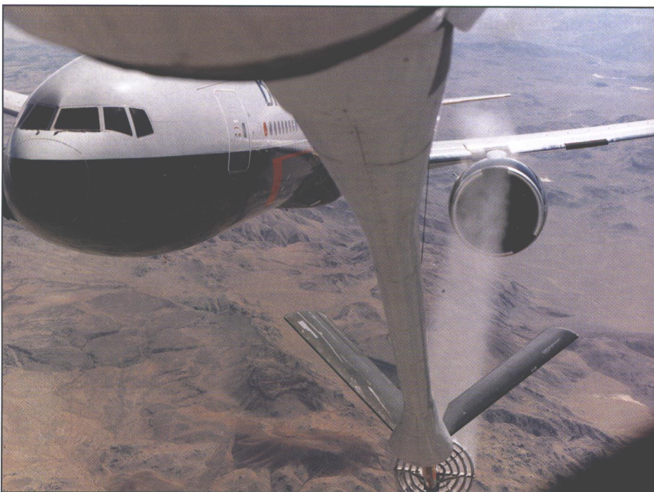
Engine icing tests on 777 WA077. Photo from the KC-135 tanker's boom operator position shows the spray array boom. Water is sprayed that becomes a controlled ice cloud due to the cold air temperature at the predetermined altitude. (Boeing/Jeff Rumsey)
