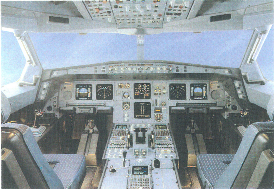
Common flight deck of the A330 (illustrated) and A340 permits crew cross-qualification 0116958
