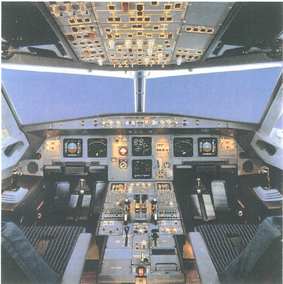
Airbus A320 flight deck with sidestick controllers outboard and six-screen EFIS NEW/0527082
