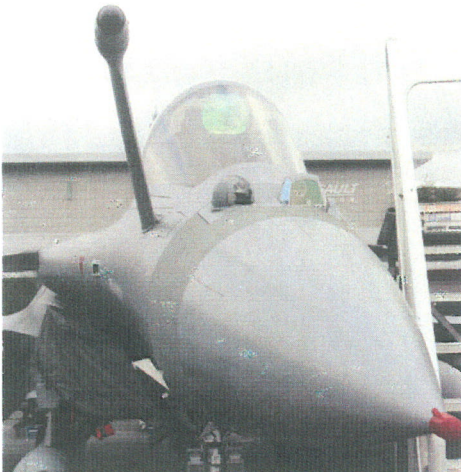
Rafale refuelling probe and OSF sensors (Paul Jackson)
