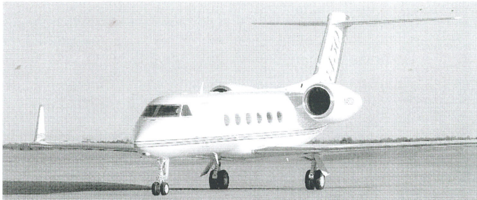
Gulfstream G450 has a longer fuselage and repositioned door, compared to G400
