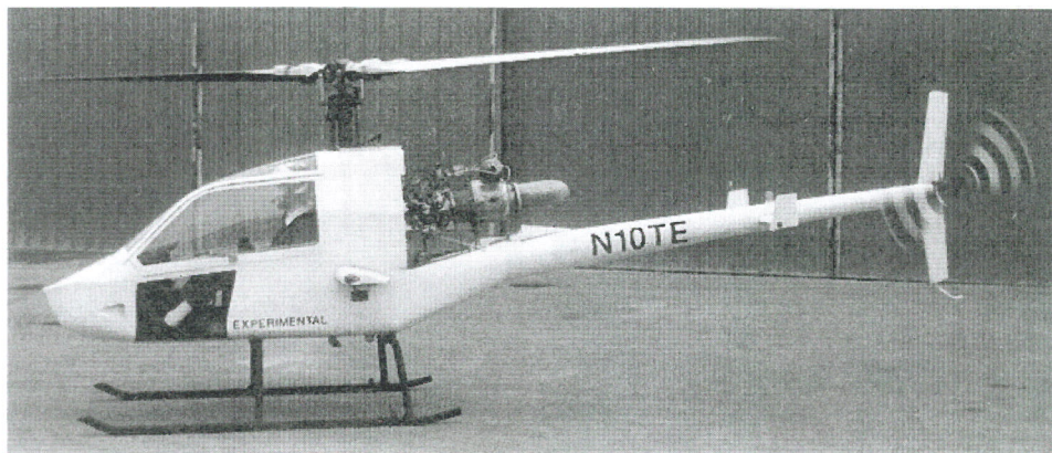
Hillberg EH 1-01 RoterMouse (one Honeywell 36-55-C)
