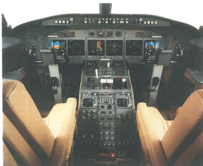
Bombardier Challenger 604 flight deck with PrecisionPlus upgraded Rockwell Collins Pro Line 4 integrated avionics
