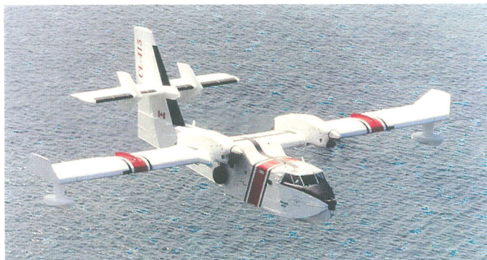
Bombardier 415 (two P&amp;WC PW123 turboprops)
