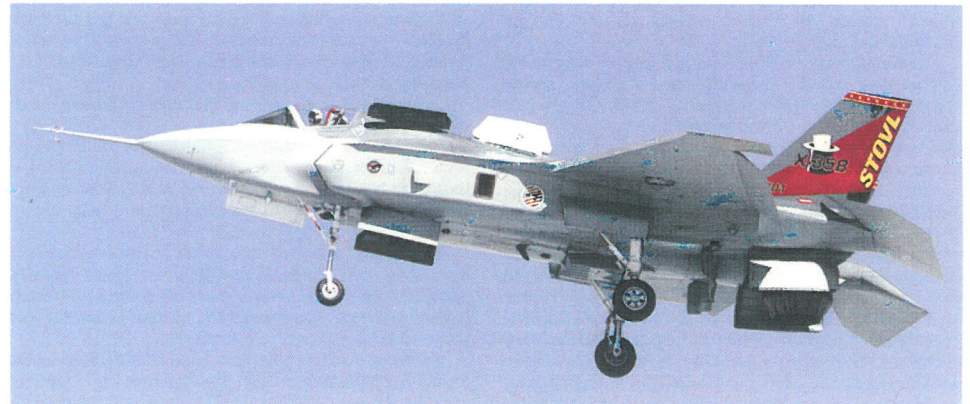
X-35B in transition mode with fan doors open and landing gear deployed
