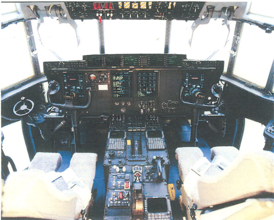
Flight deck of the C-130J, showing HUDs and EFIS
