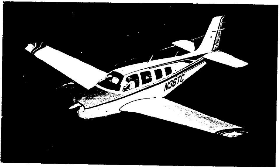
Beechcraft turbocharged Model 836TC Turbo Bonanza (Continental TSIO-520-UB flat-six engine)
