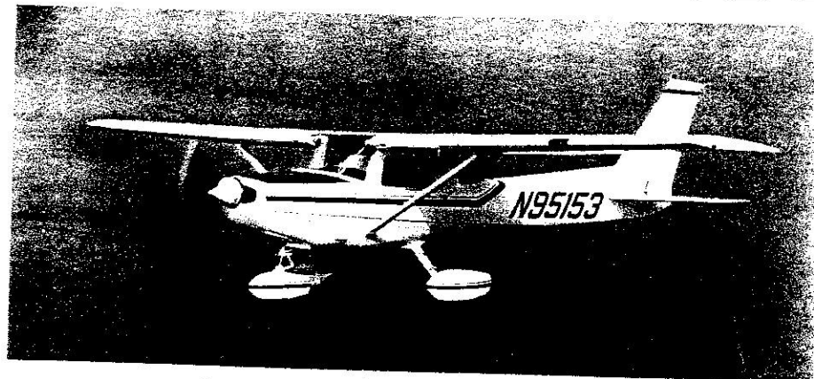
Cessna Model 152 (Avco Lycoming O-235-N2C engine)
