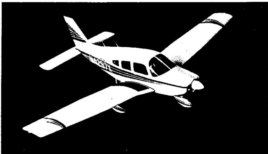
Piper Archer II, which has the tapered wings introduced on the Warrior
