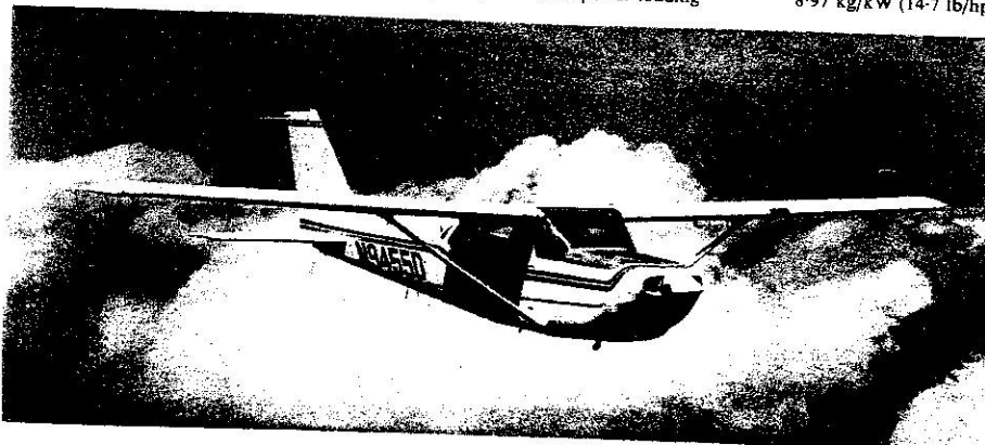
Cessna Cutlass RG four-seat lightplane with retractable landing gear
