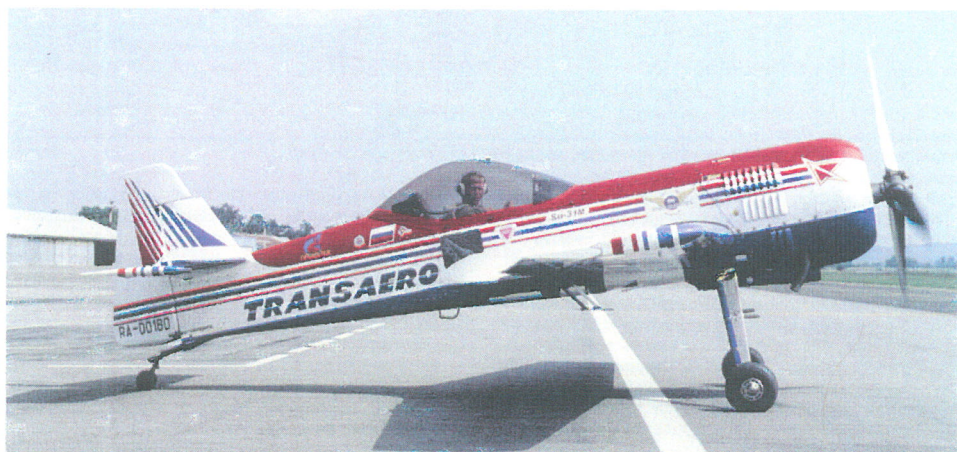
Single-piece canopy identifies the extraction system-equipped Sukhoi Su-31M (Paul Jackson)
