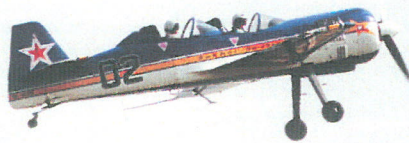
Sukhoi Su-29KS ejection system testbed, modified with separate windscreens (Yefim Gordon) 0525051
