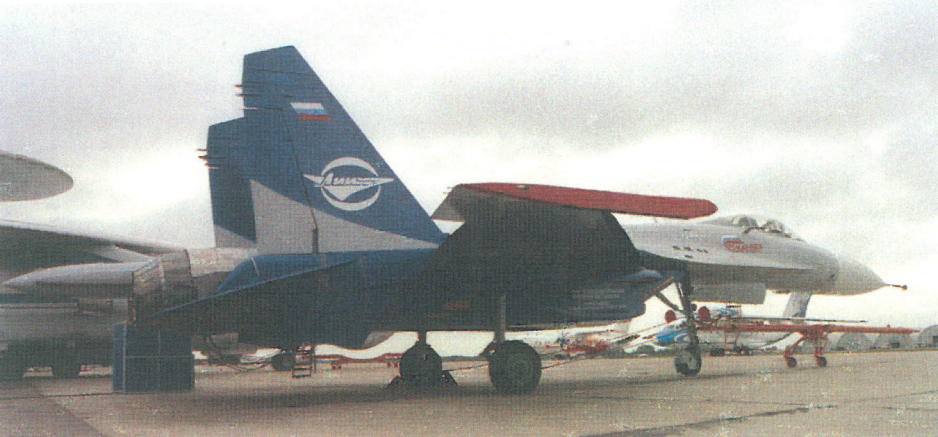
Su-27PD testbed '595' with thrust-vectoring nozzles (Yefim Gordon)
