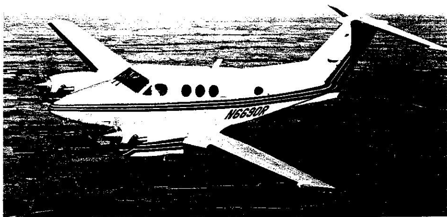
Beechcraft King Air F90-1 seven/ten-seat business aircraft, showing redesigned engine cowlings
