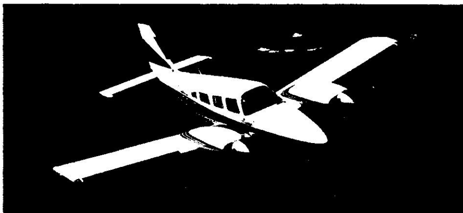
Piper Seneca III, powered by two Continental TSIO-360-KB turbocharged counter-rotating engines
