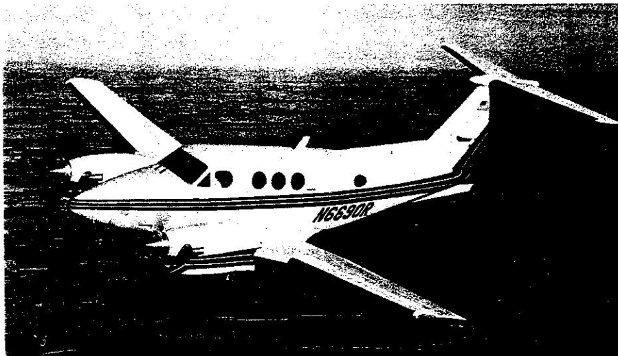
Beechcraft King Air F90-1 seven/ten-seat business aircraft, showing redesigned engine cowlings
