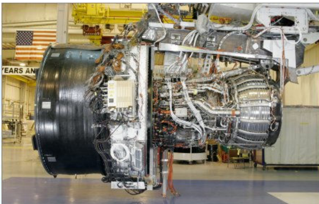
Fig.1 : Spaccati del General Electric Genx.
