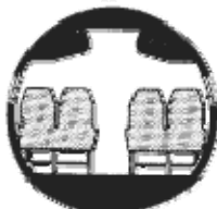
DHC-8 Aisle Height 6' 0" Max Width 8' 2"
