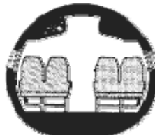
ATR-42 Aisle Height 6' 3" Max Width 8' 5"
