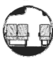
EMB-120 Aisle Height 5' 10" Max Width 7' 1"
