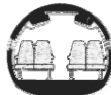
CN-235 Aisle Height 6' 2" Max Width 8' 9"
