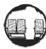
SF-340 Aisle Height 6' 0" Max Width 7' 1"
