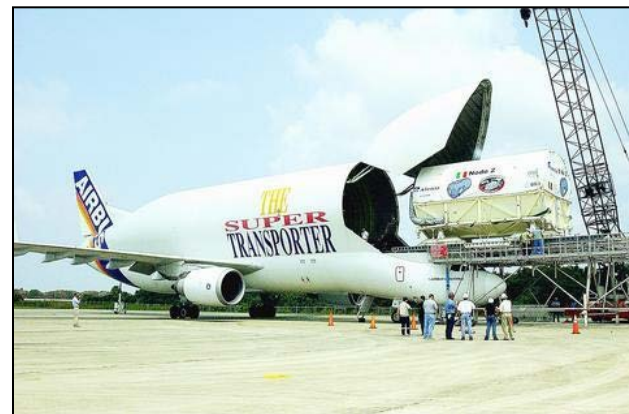
(c) Raised cockpit, visor nose
