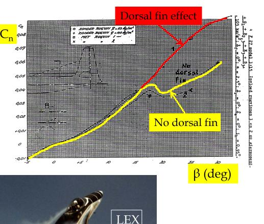
The dorsal fin exploits the same principle as the leading edge extensions (LEX) used on air superiority fighters to sustain high angles of attack
