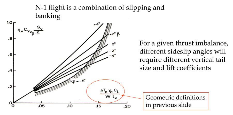
Fig. 9-22. Effect of sideslip on vertical tailplane area required to cope with engine failure
