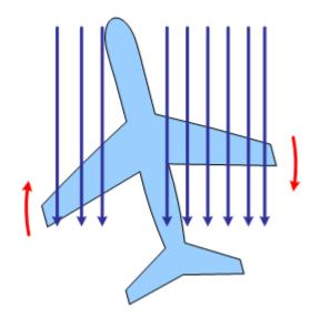
As the right wing moves forward (yaw), the sweep angle is lowered and lift increased. The aircraft will roll and then slip aside. At the same time the drag on the forward wing will increase, thereby yawing the forward wing back, hence starting the oscillations.
