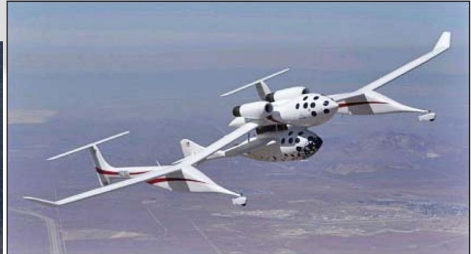
The Scaled Composites Model 318 White Knight is a jet-powered carrier aircraft used to launch the [SpaceShipOne](#) experimental spacecraft. It was developed by Scaled Composites as part of their Tier One program.
