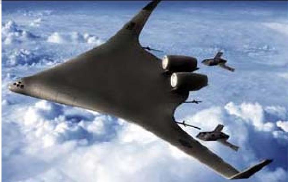
**Fig. 3.8** The flying-wing layout.
