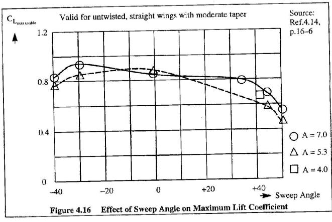
The trend is for the useful wing  $C_{L_{mex}}$  to decrease with increasing aft sweep in the moderate sweep angle range of +/-25 degrees. Initially, this decrease follows the cosine-rule of Ref. 4.15, page 339):
