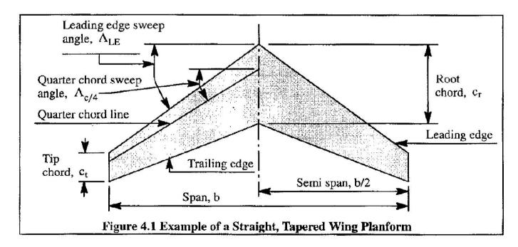
The wing area, S is defined as the shaded area in Figure 4.1. In general, S is defined as the area of the wing planform, projected onto a plane of reference which is usually the wing root chord plane.
