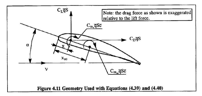
$$C_{m_{ac}}\overline{q}S\overline{c} = C_{m_{x}}\overline{q}S\overline{c} + C_{L}\overline{q}S(x_{ac} - x)\cos\alpha + C_{D}\overline{q}S(x_{ac} - x)\sin\alpha \qquad (4.37)$$
