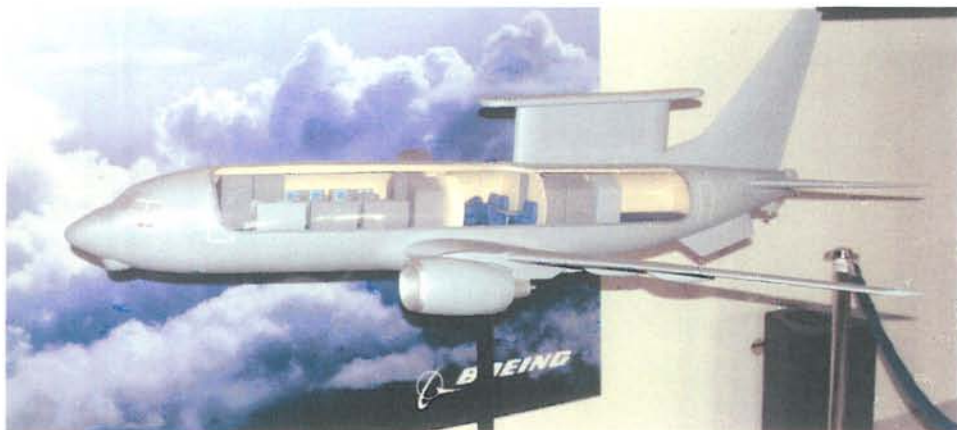
Cutaway model of Boeing 737 AEW&amp;C variant adopted by Australia (Paul Jackson)
