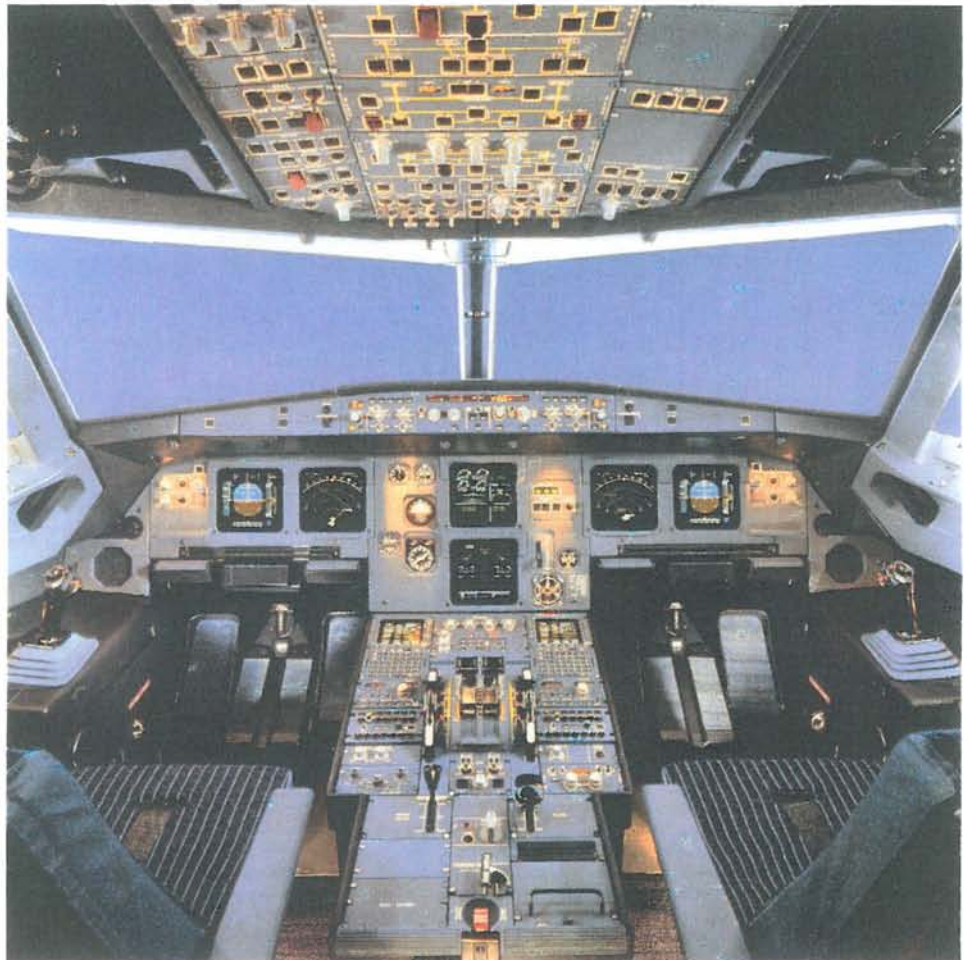
Airbus A320 flight deck with sidestick controllers outboard and six-screen EFIS
