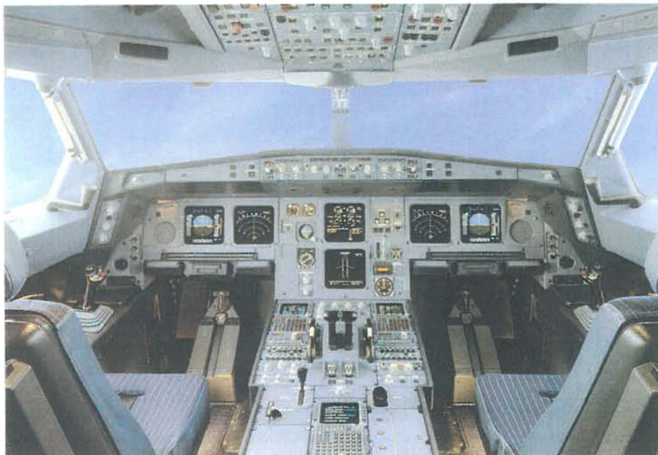
Common flight deck of the A330 (illustrated) and A340 permits crew cross-qualification
