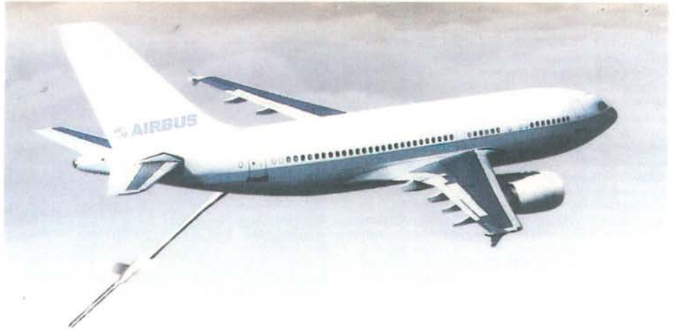
Computer-generated image of an A310 MRTT with 'flying boom' equipment
