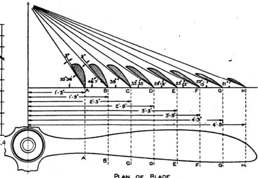
FIG. 219.—Lay-out of an Aircsrew.
