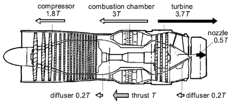
Figure 5.21 Distribution of internal thrust components for a static turbojet.
