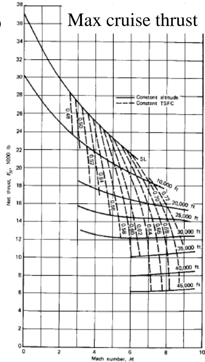
**Figure 6.38** JT9D-7A maximum cruise thrust. One hundred percent ram recovery, no airbleed, no power extraction, Pratt & Whitney Aircraft reference exhaust system, all curves for ICAO standard day +10°C and below. (Courtesy, Pratt & Whitney.)
