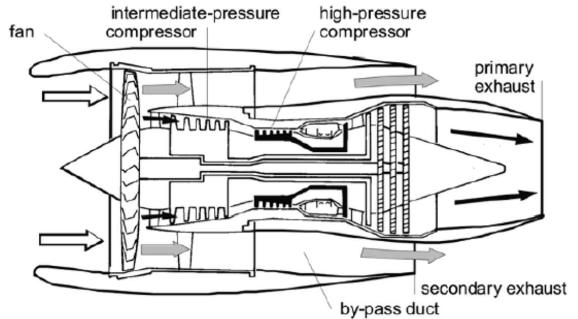
(b) Three-shaft high by-pass ratio turbofan
