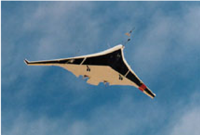
BWB-17 NASA-Stanford, 1996 5.2 m span scaled model flight
