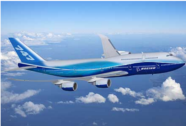
B747-800 Stretched fuselage New engines (B787) Fly-by-wire
