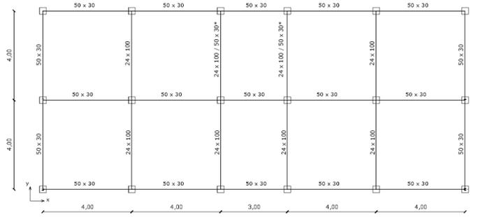
Figure 1: Storey view (dimensions in m) *Beam frame labels indicate the section dimensions in cm; column sections are all (30x30) \*this frame represents both storey beams (24x100) and stair knee beams (50x30)*
