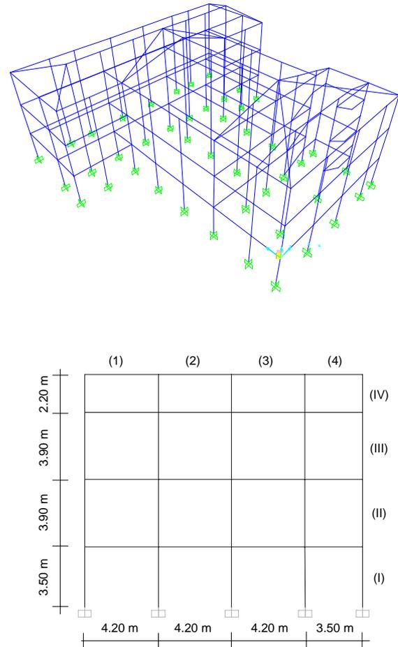
Figure 5(a) The tri-dimensional view of the scholastic building 5(b) The central frame of the case-study building
