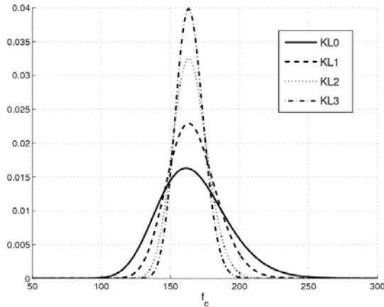
Figure 1. The prior and the updated probability distributions for concrete for different knowledge levels.
