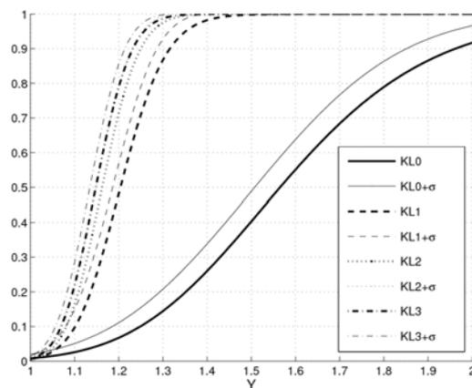
Figure 6 The structural fragility curves for the knowledge levels KL<sub>0</sub>, KL<sub>1</sub>, KL<sub>2</sub> and KL<sub>3</sub>.
