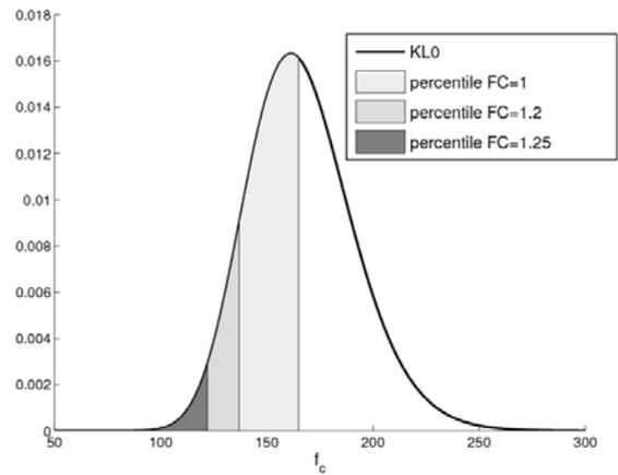
Figure 3 The percentiles corresponding to each CF on the prior probability distribution for concrete.
