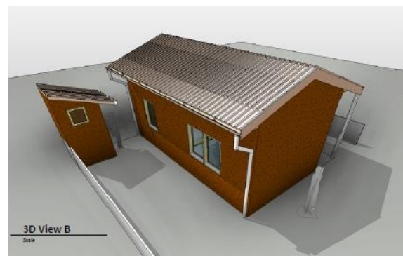
Figure 14 – The elevation (a) and 3d (b) view sketches of a mud and wood structure with water-proof roof system. Note the position of drains and the inclination of the roof (drawings courtesy of EiABC)
