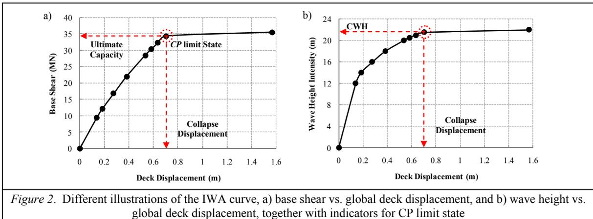
Figure 2. Different illustrations of the IWA curve, a) base shear vs. global deck displacement, and b) wave height vs. global deck displacement, together with indicators for CP limit state
