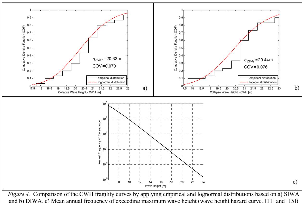
Figure 4. Comparison of the CWH fragility curves by applying empirical and lognormal distributions based on a) SIWA and b) DIWA, c) Mean annual frequency of exceeding maximum wave height (wave height hazard curve, [11] and [15])
