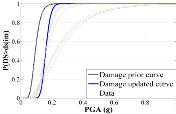
Figure 3 Damage fragility curves.
