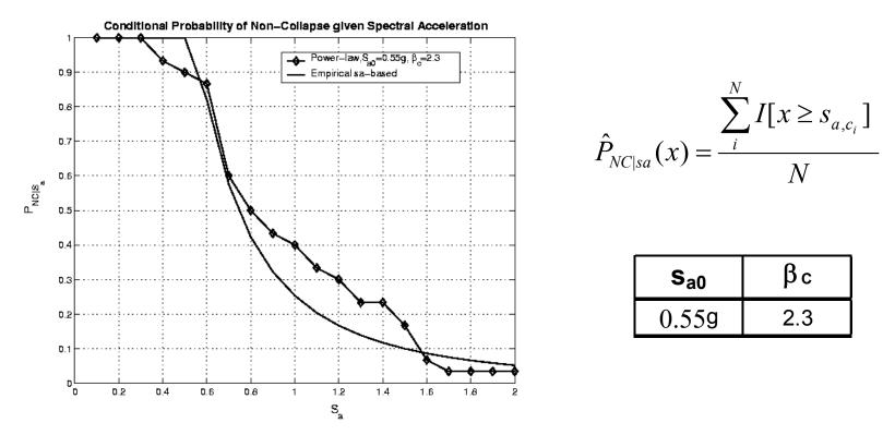
The probability of non-collapse is estimated by the ratio of the collapsed to
