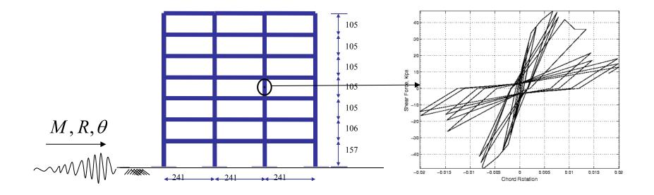
Beam-column model with stiffness and strength degradation in shear and flexure using DRAIN2D-UW by J. Pincheira et al.
