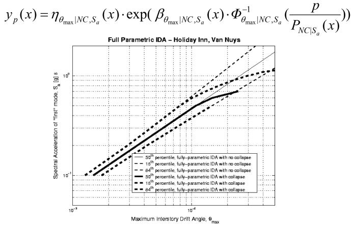
The 16th, 50th, and 84th percentiles for the three-parameter distribution are plotted as functions of spectral acceleration.
