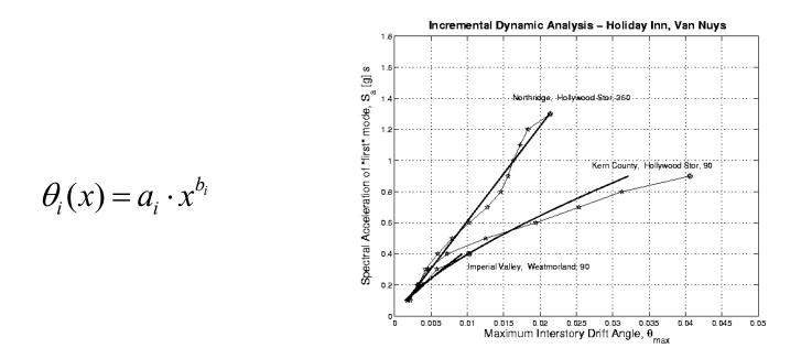
IDA curves in the non-collapse regime approximated by power-law functions. The points marked as circles in the end are the points at which the global instability capacity was reached.
