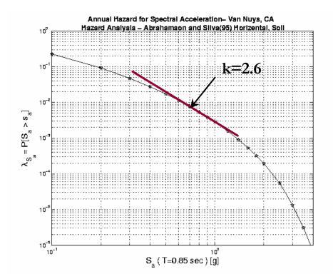
Site-specific hazard curve, Van Nuys CA, and a linear approximation to the hazard curve.
