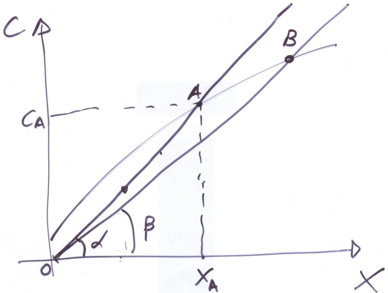
$$c = \frac{C}{X} = \frac{\overline{OC_A}}{\overline{OX_A}} = \frac{\overline{X_A A}}{\overline{OX_A}}$$
