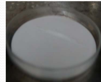
Microcapillary are left dry overnight and transferred in oven a 60-80 ^{\circ}\text{C}
