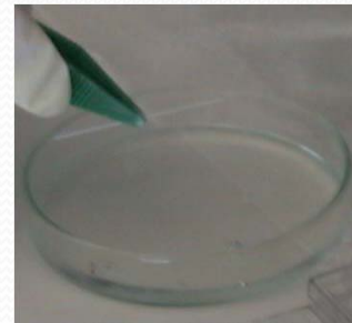
microcapillary glass are gently placed in a silicizing solution (dimethyldichlorosilane in chloroform)
