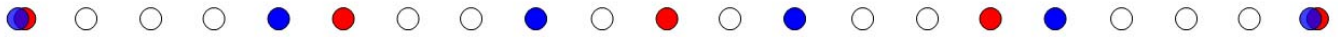
Figure 1. CopSAR concept, N_1=4 , N_2=5 : locations along the SAR line of flight at which pulses are transmitted. Blue: first sequence; red: second sequence; white: pulse not transmitted.
