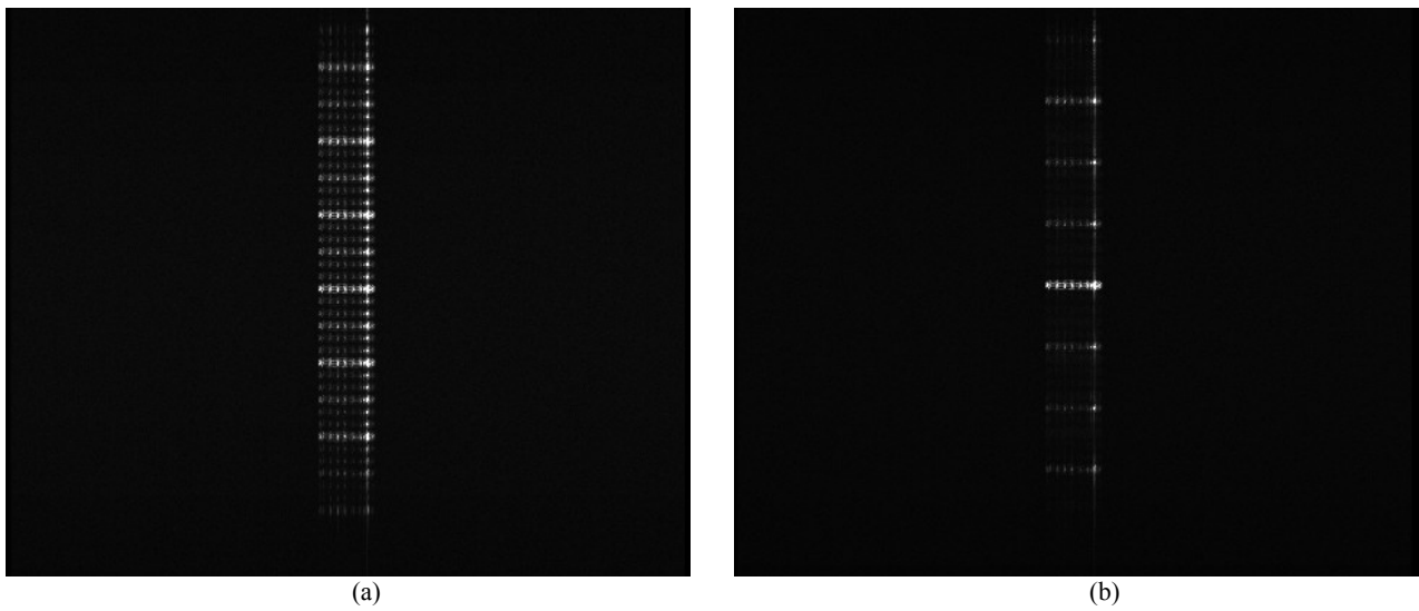
Figure 11. CopSAR missing-pulse implementation, N_1=5 and N_2=6 : simulated image s_1(x,r) (a) and the associated CopSAR image (b). A 4x4 multilook is applied.
