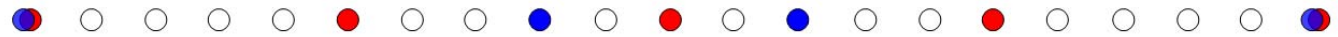
Figure 2. CopSAR concept, N_1=4 , N_2=5 , “missing-pulse” implementation: locations along the SAR line of flight at which pulses are transmitted. Blue: first sequence; red: second sequence; white: pulse not transmitted.
