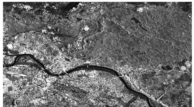
Fig. 8. Fragment of the Sentinel-1 acquisition of Dresden city. The image has been processed up to 15 ENL using spatial multilooking and multitemporal despeckling. It has a spatial resolution of about 15 m. The original patch size is about 1000 \times 1700 pixels.
