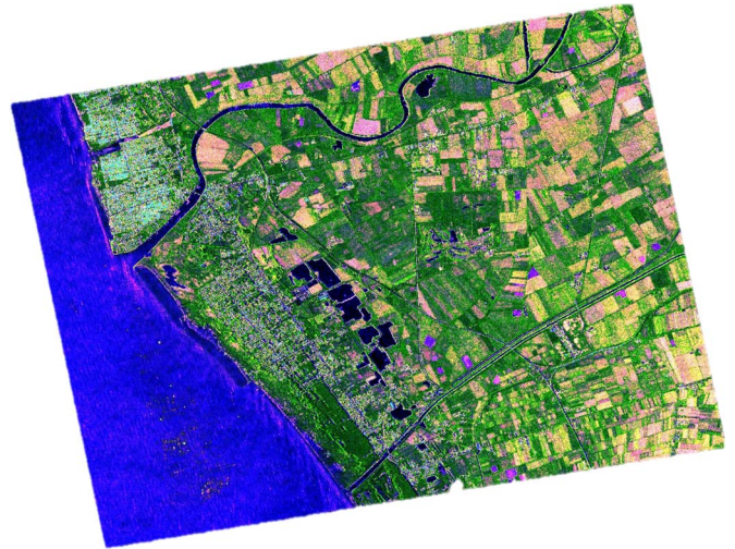
Fig. 4. Campania data set: summery Level-1 \beta product obtained by processing eight images from April to October 2010. Roughly, the following color-object association can be made: blue—sea, black—stagnant water/weak scatterers, green—grasslands/unchanged land cover, cyan—urban area/built-up, and yellow/pink—growing vegetation. The original image dimension is about 4400 × 5000 pixels.
