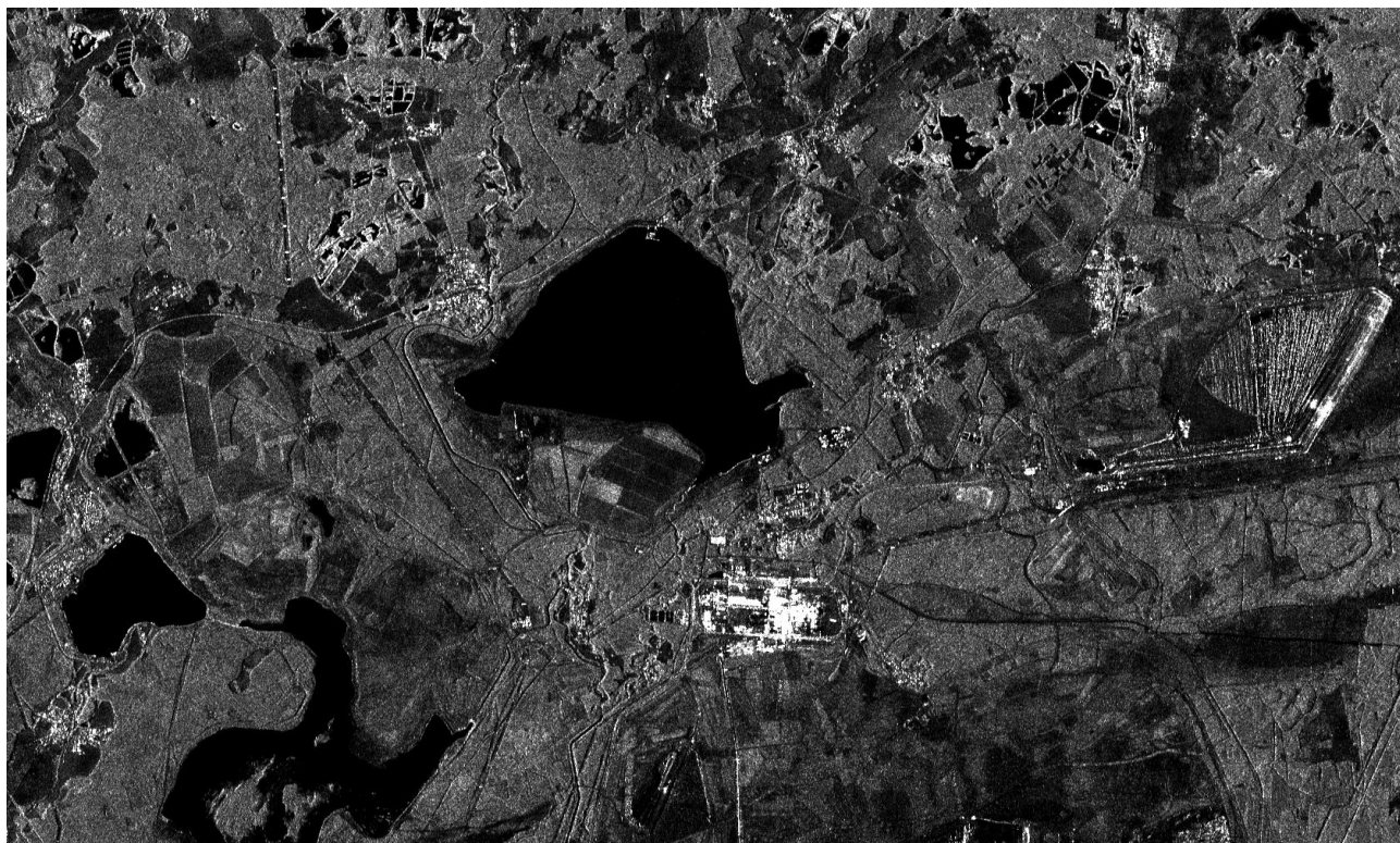
Fig. 2: A small portion of one of the available Sentinel-1 images with 15 meters spatial resolution processed up to 15 ENL.
