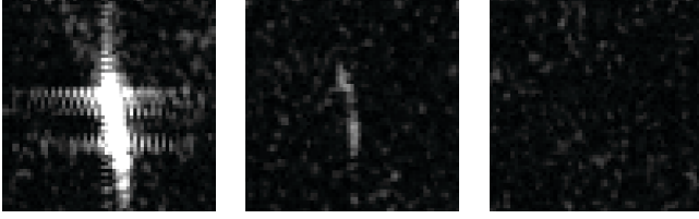
Fig. 1. Examples of patches with, from left to right, ship, ghost (replica of the previous ship), and sea.
