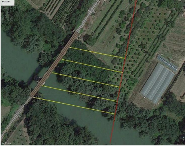
Fig.1 SAR acquisition geometry: the line of flight of the sensor is represented in red.
