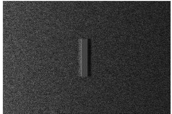
Figure 1. Simulated SAR image relative to a single building on a rough surfaces. Main simulation parameters are provided in the first line of Table II. Near range is on the left.
