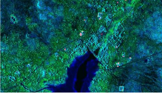
Fig. 1: Burkina Faso, Level-1 \alpha product. Blue band: dry season image. Green band: wet season image.
