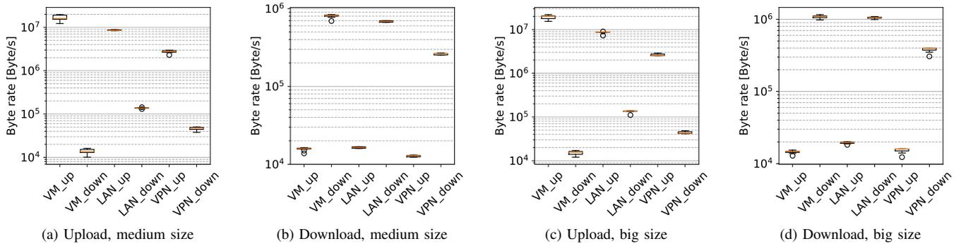
Fig. 4: Average byte rate over the total duration of transfer. Medium and Big sizes are for 100MB and 1GB, respectively.
