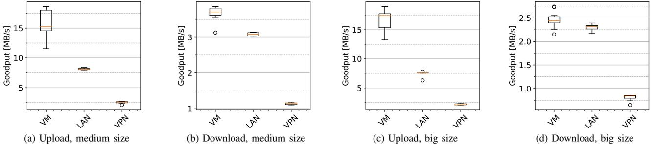
Fig. 3: Goodput (ratio of Images Set total size over the total duration of transfer). Medium and Big sizes are for 100MB and 1GB, respectively.
