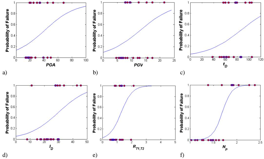
**Figure 3.2.** Comparing probability of failure in terms of  $D_\gamma$  using logistic regression for frame F10 at a fixed  $Sa(T_1)=1500\text{cm/s}^2$  versus a)  $PGA$ ; b)  $PGV$ ; c)  $t_D$ ; d)  $I_D$ ; e)  $R_{T1,T2}$  and f)  $N_p$
