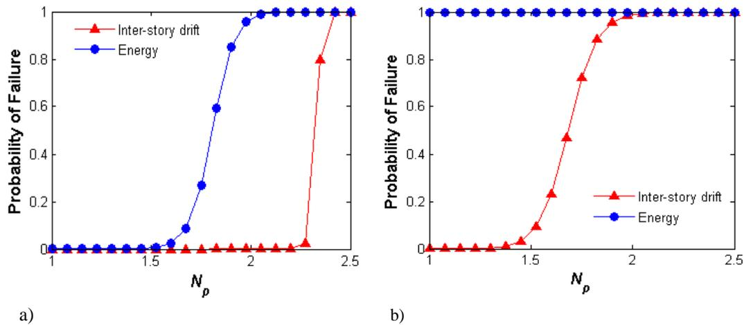
**Figure 3.4.** Probability of failure for  $D_\gamma$  versus  $D_{EN}$  for frame F8 at a fixed a)  $Sa(T_1)=900\text{cm/s}^2$ ; b)  $Sa(T_1)=1500\text{cm/s}^2$
