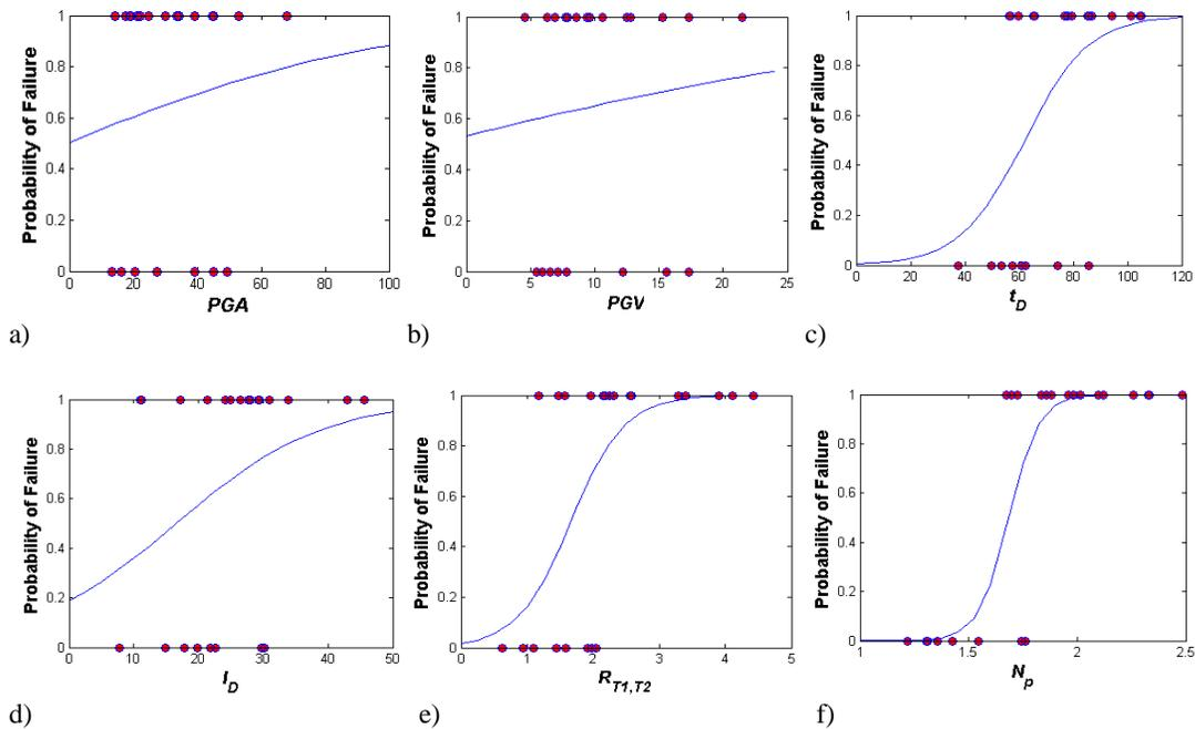
**Figure 3.1.** Comparing probability of failure in terms of  $D_\gamma$  using logistic regression for frame F8 at a fixed  $Sa(T_1)=1500\text{cm/s}^2$  versus a)  $PGA$ ; b)  $PGV$ ; c)  $t_D$ ; d)  $I_D$ ; e)  $R_{T1,T2}$  and f)  $N_p$
