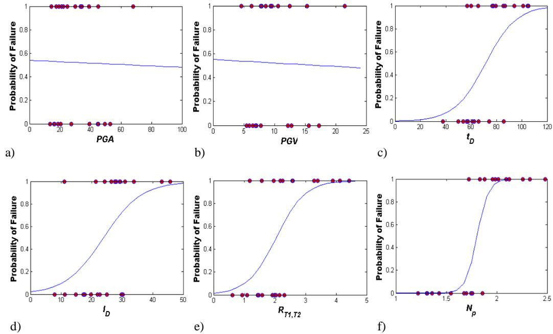
**Figure 3.3.** Comparing probability of failure in terms of  $D_{EN}$  using logistic regression for frame F8 at a fixed  $Sa(T_1)=900\text{cm/s}^2$  versus a)  $PGA$ ; b)  $PGV$ ; c)  $t_D$ ; d)  $I_D$ ; e)  $R_{T1,T2}$  and f)  $N_p$
