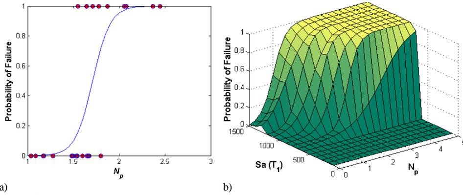
**Figure 2.1.** a) Logistic regression for a fixed spectral acceleration and the vector  $\langle Sa(T_1), N_p \rangle$ ; b) probability of failure versus,  $Sa(T_1)$  and  $N_p$
