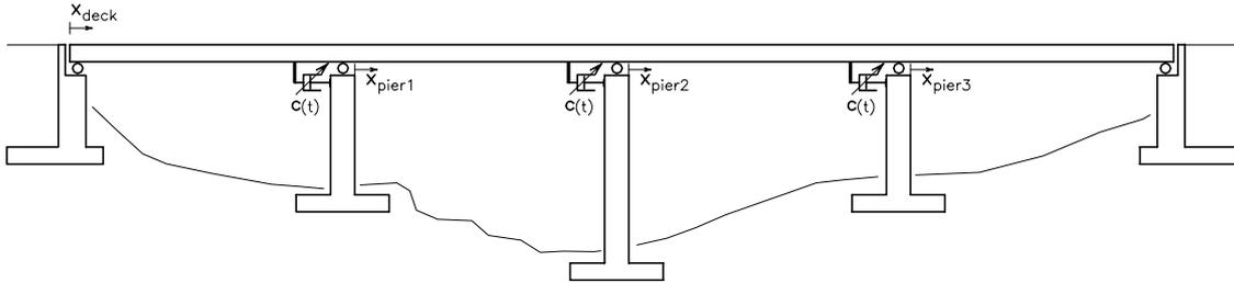
Figure 3. Isolated viaduct with variable-constant dampers
