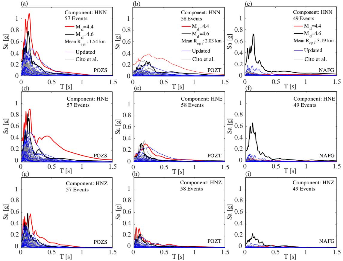
Figure 3. Pseudo-acceleration (5% damped) response spectra at POZS (a,d,g) POZT (b,e,h) and NAFG (c,f,i) stations. Panels a-f refers to the horizontal components of ground motions, while panels g-i represent spectra for vertical component. (The spectra for the  $M_d = 4.4$  event and that for  $M_d = 4.6$  are plotted in red and black, respectively, to distinguish.)
