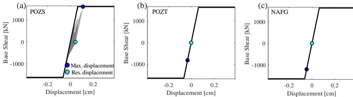
Figure 7. ESDoF system of the URM structure subjected to the accelerograms from the  $M_d \geq 2.5$  earthquakes recorded at POZS (a), POZT (b), and NAFG (c) stations.
