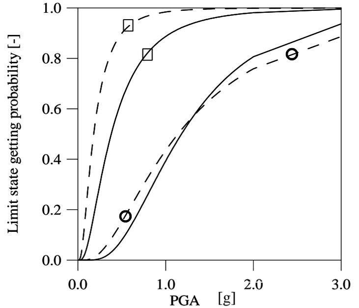
Figure 3. Experimental fragility curves for atmospheric steel tanks affected by earthquakes. Dotted line represents tank fill level > 50%. □: RS2; ○: RS3.
