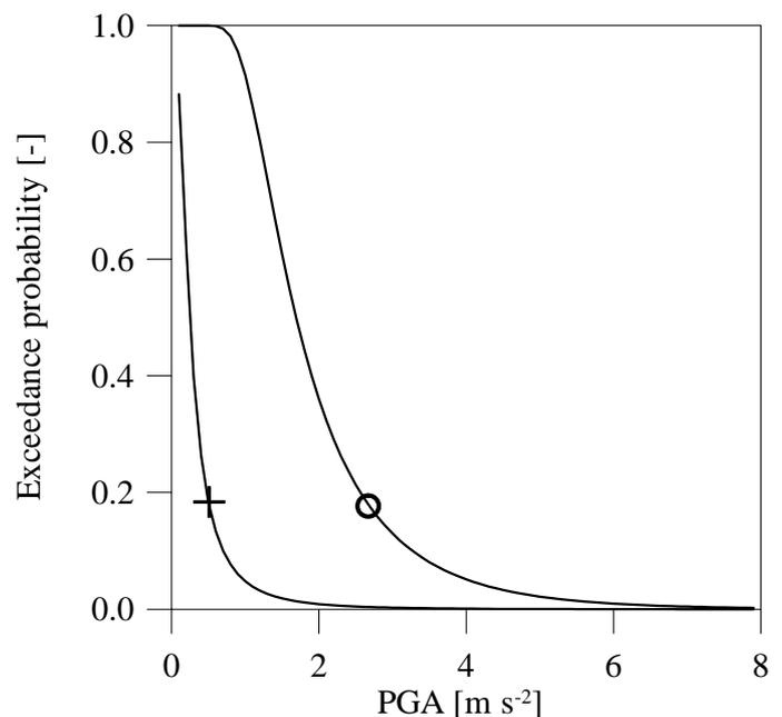
Figure 1. Hazard curves in terms of annual exceedance probability of Peak Ground Acceleration (PGA) for two equipment with service life of respectively: + : 50 year; O: 1 year
