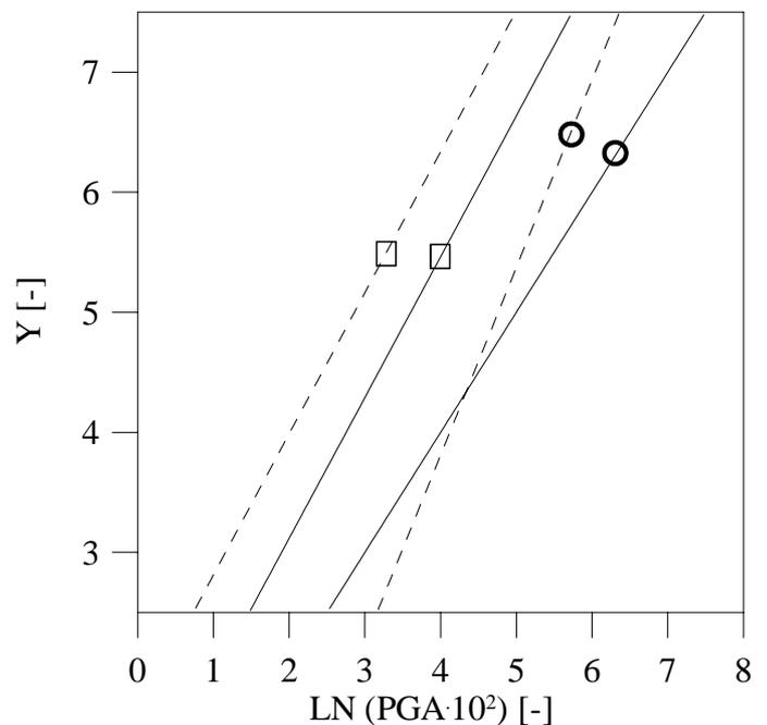
Figure 4. Probit analysis for steel tanks in seismic areas. Dotted line represents tank fill level > 50%. □: RS2; ○: RS3.
