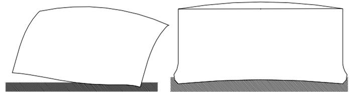
Figure 2. Unanchored atmospheric tank subjected to "uplifting" and "elephant foot" buckling.
