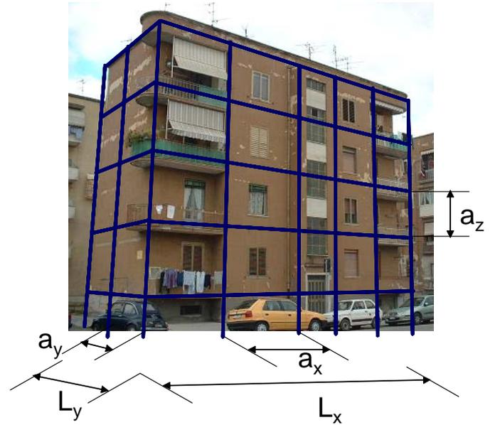
Figure 1. Typical R.C. building generated.
