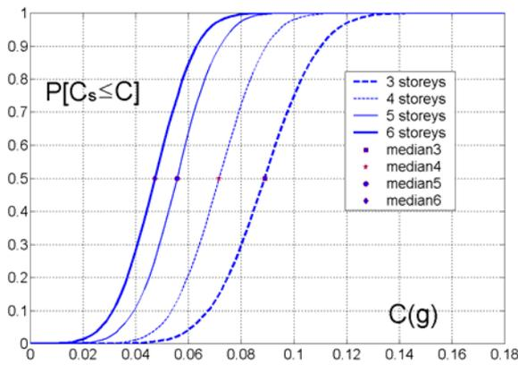
Figure 5.  $C_s$  capacity curve for 3, 4, 5 and 6 storey classes.
