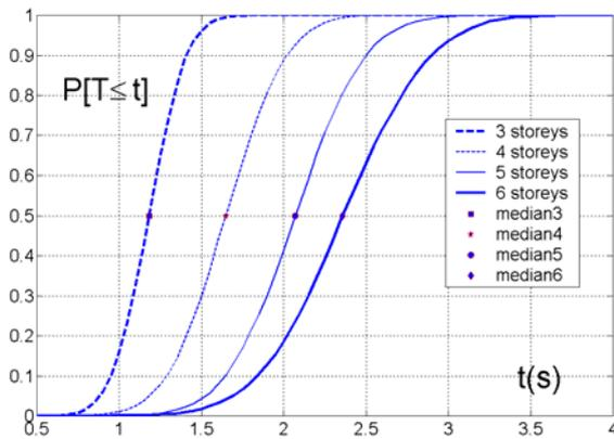
Figure 6.  $T$  curve for 3, 4, 5 and 6 storey classes.
