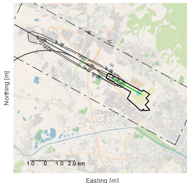
Fig. 16. Individual risk (annual fatality probability contours for the 2029 traffic scenario of the upgraded Amerigo Vespucci airport.
