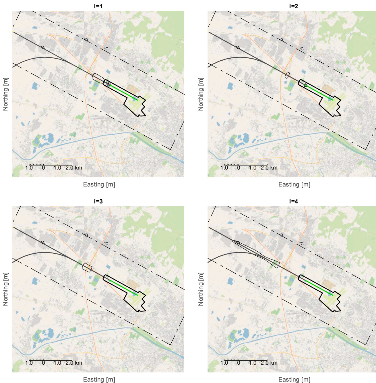
Fig. 11. Contours of annual rates of leakage in the Amerigo Vesupucci airport area during takeoff.
