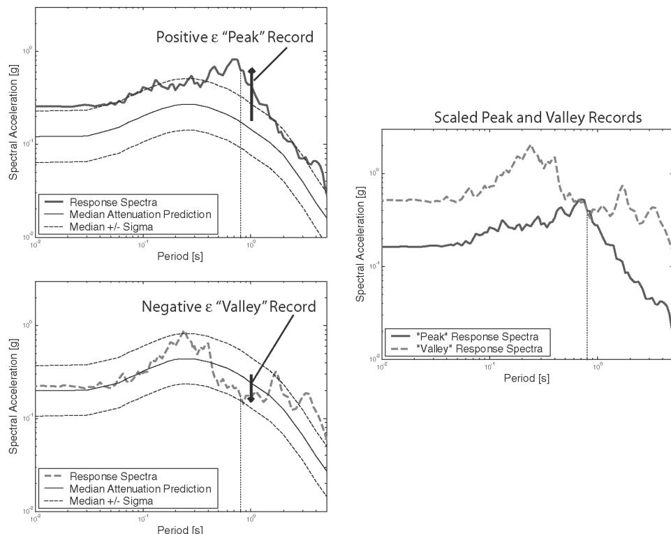
**FIGURE 1** Scaling a negative  $\varepsilon$  record and a positive  $\varepsilon$  record to the same spectral acceleration at the period of 0.8 s. Courtesy of Jack W. Baker; see Baker and Cornell [2005] for details.
