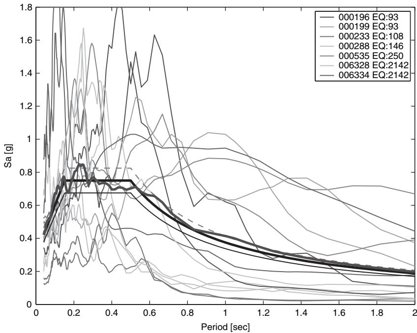
**FIGURE 7** Site class B – Zone 2. Set with minimum average deviation from the target spectrum ( $\delta = 0.07$ ) and minimum single-record deviation from the target ( $\delta_{\max} = 1.0$ ).
