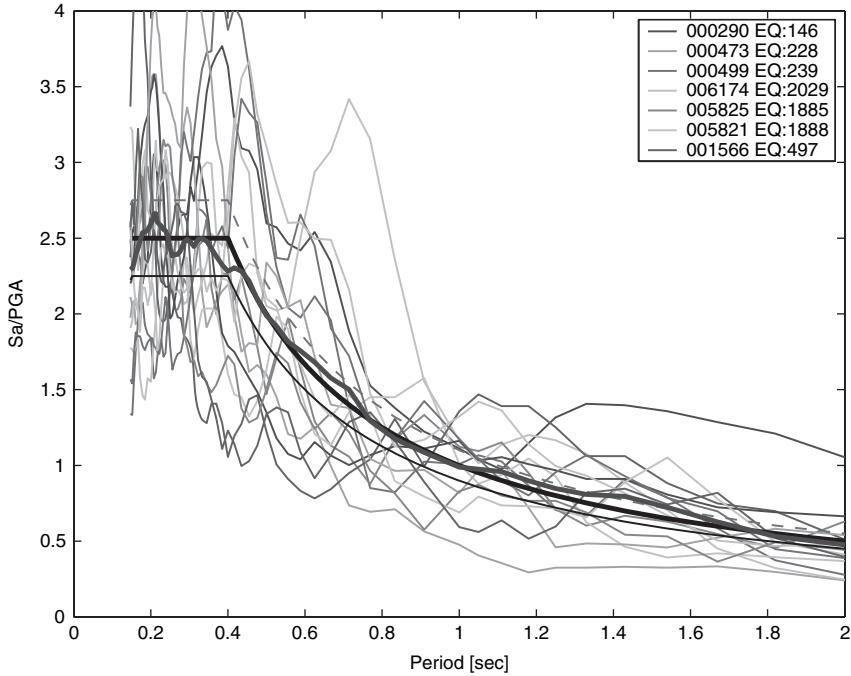
**FIGURE 21** Site class A – S-type. Set with minimum average deviation from the target spectrum ( $\delta = 0.047$ ) with records coming from seven different events.
