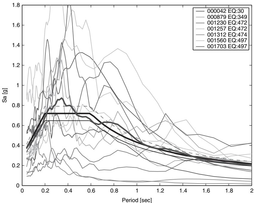
**FIGURE 10** Site class C – Zone 2. Set with minimum average deviation from target spectrum ( $\delta = 0.08$ ).
