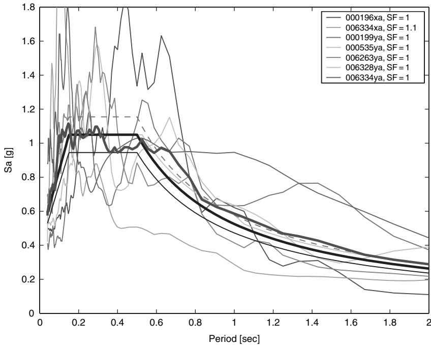
**FIGURE 17** Site class B – Zone 1. Set with minimum average deviation from target spectrum ( $\delta = 0.07$ ). SF is the individual scale factor.
