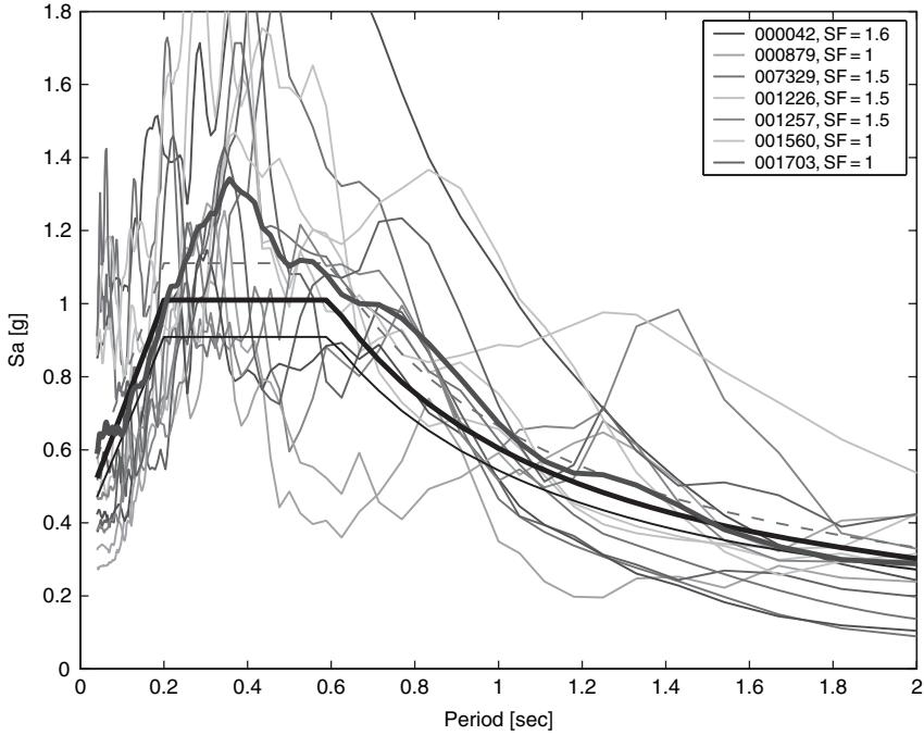
**FIGURE 11** Site class C – Zone 1. Set with minimum average deviation from target spectrum ( $\delta = 0.173$ ). SF is the individual scale factor.
