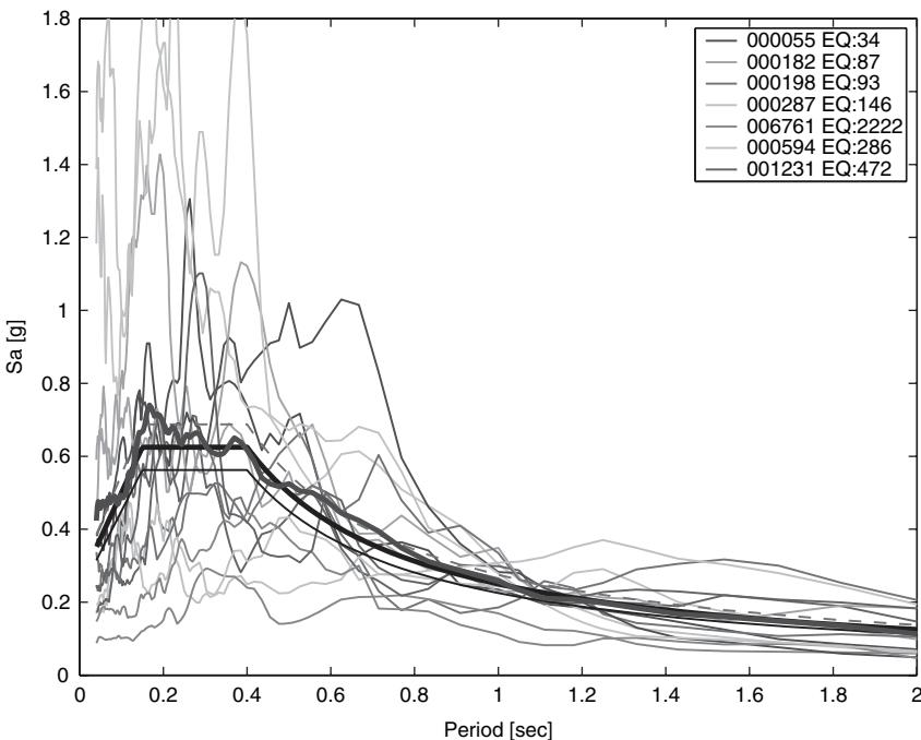
**FIGURE 4** Site class A – Zone 2. Set with minimum average deviation from target spectrum ( $\delta = 0.122$ ) with records coming from seven different events.
