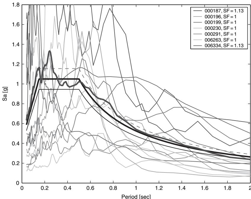
**FIGURE 8** Site class B – Zone 1. Set with minimum average deviation from target spectrum ( $\delta = 0.07$ ). SF is the individual scale factor.
