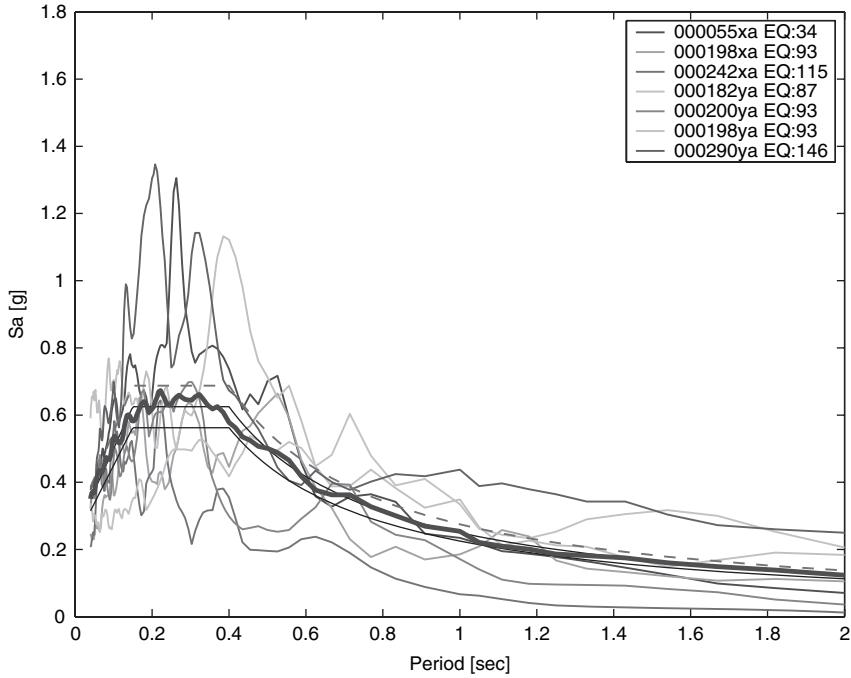
**FIGURE 13** Site class A – Zone 2. Set with minimum average deviation from the target spectrum ( $\delta = 0.04$ ) and minimum single-record deviation from the target ( $\delta_{\max} = 0.51$ ).
