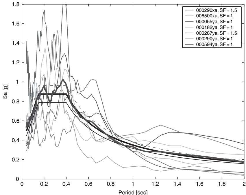
**FIGURE 14** Site class A – Zone 1. Set with minimum average deviation from target spectrum ( $\delta = 0.1$ ). SF is the individual scale factor.
