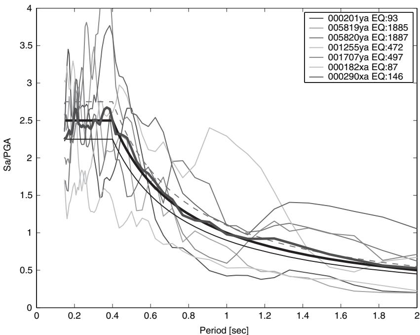
**FIGURE 22** Site class A – P-Type. Set with minimum average deviation from the target spectrum ( $\delta = 0.058$ ) with records coming from seven different events.
