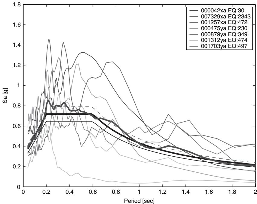
**FIGURE 19** Site class C – Zone 2. Set with minimum average deviation from the target spectrum ( $\delta = 0.08$ ) and minimum single-record deviation from the target ( $\delta_{\max} = 0.54$ ).
