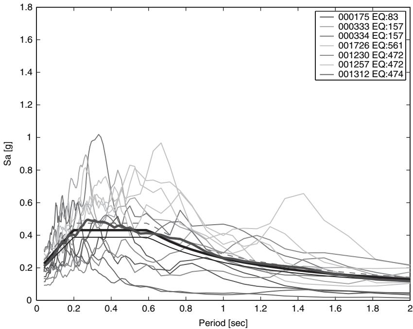
**FIGURE 9** Site class C – Zone 3. Set with minimum average deviation from the target spectrum ( $\delta = 0.07$ ) and minimum single-record deviation from the target ( $\delta_{\max} = 0.572$ ).
