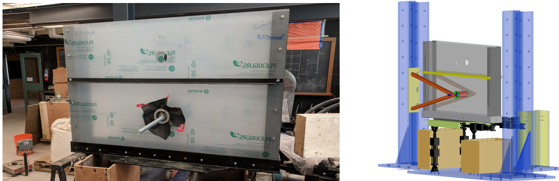
Figure 4: Overview of the experimental setup at the University of Toronto to study the soil-pipeline system static stiffness and detail of the soil-pipe box to be tested (bottom).
