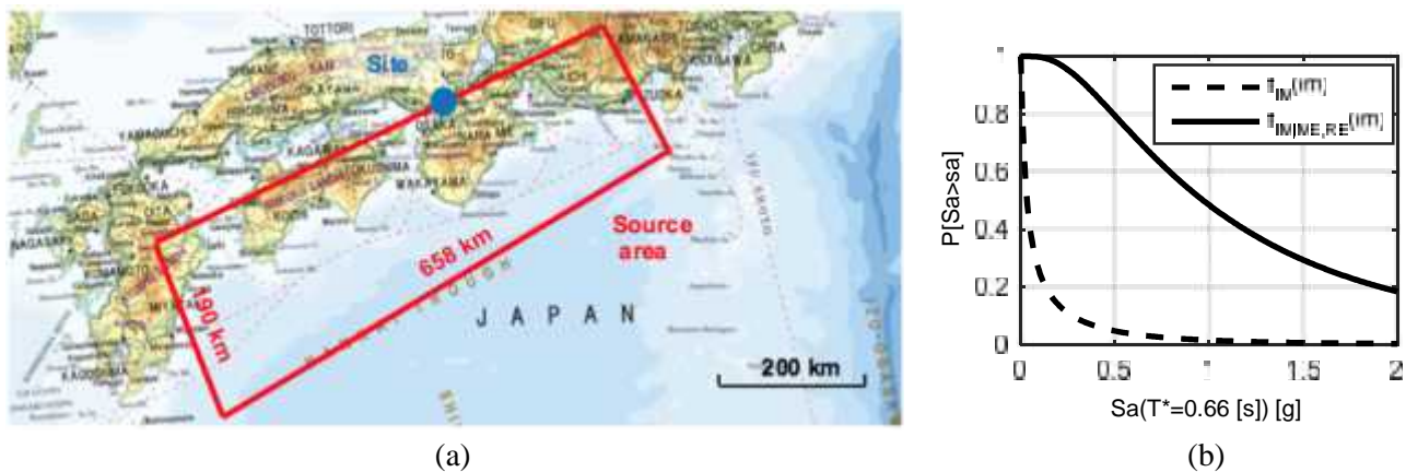
Fig. 5 – APSHA results; (a) site and source zone; (b) the probability distribution of IM exceedance in one aftershock event, f_{IM} , and the probability distribution of IM exceedance for the mainshock of given magnitude and source-to-site distance, f_{IM|M_E, R_E} .
