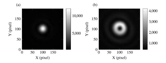
FIG. S1. Spatial mode images of single down-converted photons taken with an electron multiplying charge coupled device (EMCCD) camera. Only one photon of each pair is selected with a linear polarizer after the non-linear crystal. (a) Profile of the Gaussian mode before the q-plate transformation and (b) the orbital angular momentum eigenstate after passing through the q-plate.
